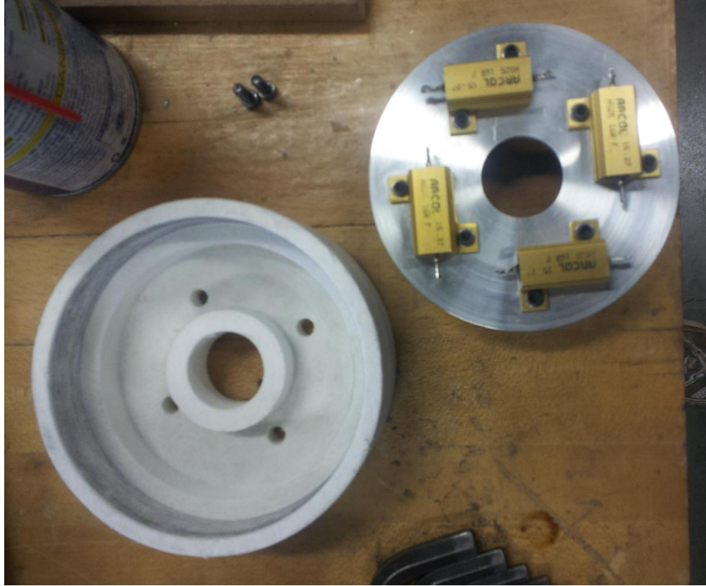
Heat spreader (bottom) thermal isolator (top)
