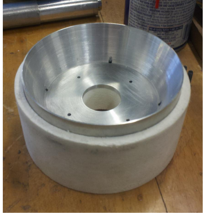
Heat spreader inside thermal isolator
