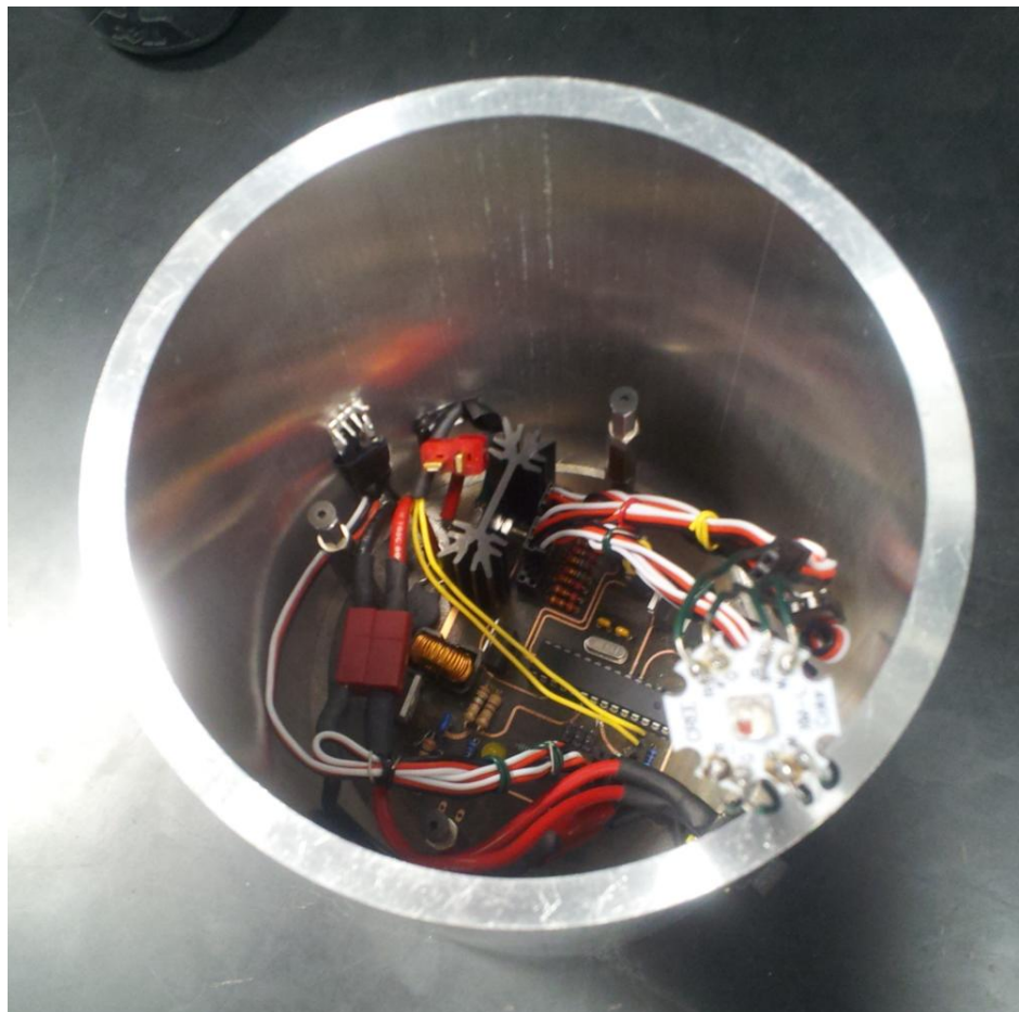
PCB et. al. mounted inside of the shell
