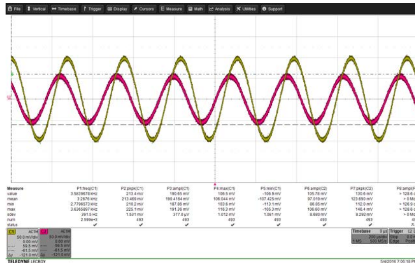
Figure 22: Summing-Inverting amp at 3.6 kHz Input signal level (Yellow): 213 mV pp Output signal level (Pink): 123 mV pp
