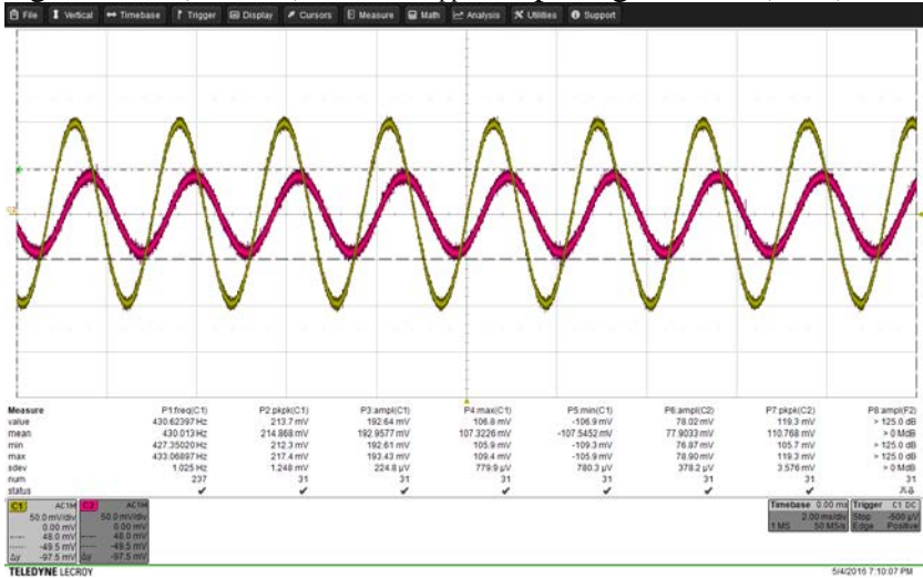
Figure 20: Summing-Inverting amp at 430 Hz Input signal level (Yellow): 215 mV pp Output signal level (Pink): 111 mV pp
