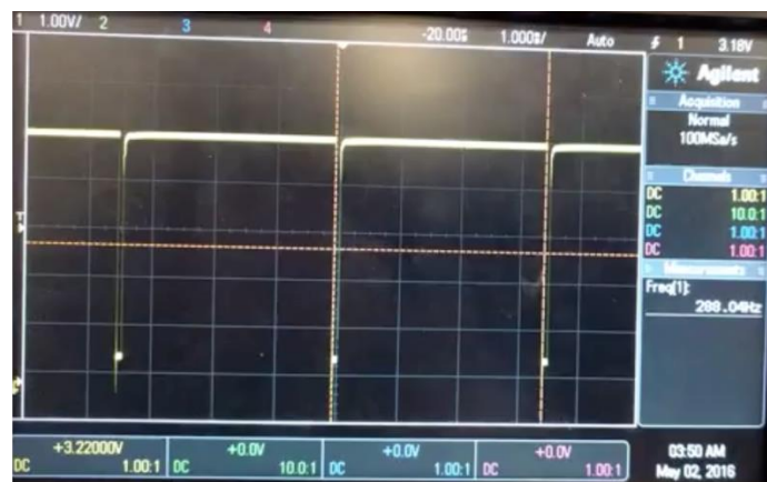
Figure 15: PWM Output from Timer (LM 555) at Duty Cycle 100% vs Time
