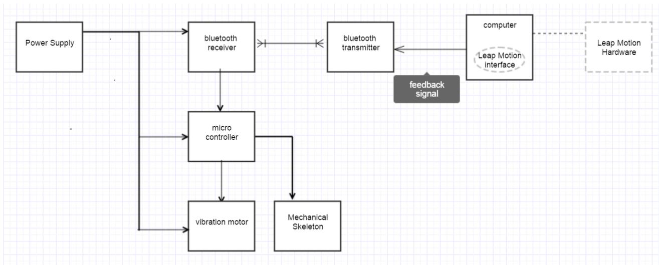
Figure 1: High Level Block Diagram of the Glove
