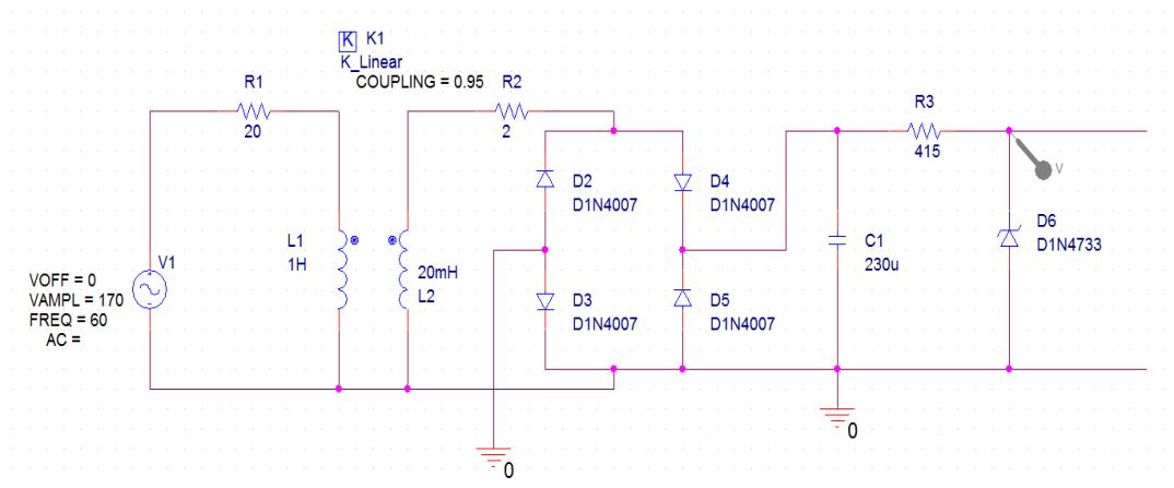
Since the lowered voltage still stands at  $15\text{V}_{\text{rms}}$ , and the desired voltage is  $5\text{V}$ , we employ a regulator, in this case a zener diode in series with a resistor. We use 1N4733 for the zener diode, which provides us with  $5.1\text{V}$  zener voltage. To obtain the resistance required to achieve our goal, we calculate it as follows:
