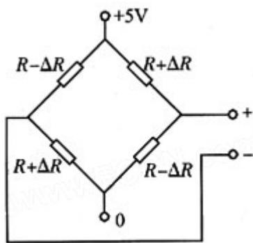
Assume we have the relationship between pressure and resistance  $R=kP$  ( $k$  is constant) then  $\Delta R=k\Delta P$  so the output voltage of the bridge should be  $((R+\Delta R)/2R - (R-\Delta R)/2R) \cdot U = \Delta R/R \cdot U = k \cdot \Delta R/R \cdot U$ . If we set  $R_1/R_4 = R_2/R_3$  and  $R_6/R_7 = R_5$ , we will get our output voltage  $U_{out} = k \cdot \Delta P \cdot U / R \cdot R_3 / R_2 \cdot R_7 / R_6$  which will be sent to our microcontroller.
