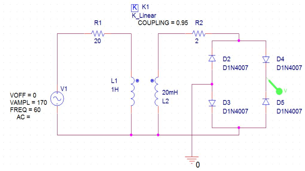
To rectify the alternating current, we intend to take advantage of the feature of diodes. Here, we use the bridge rectifier since it is more efficient than the half-wave circuit or the center-tapped full-wave circuit. Specifically, we use four 1N4007 diodes, from Vishay Semiconductor Diodes Division, to realize that purpose. Since the current can only go under forward-biased condition, the output current will be positive as desired.
