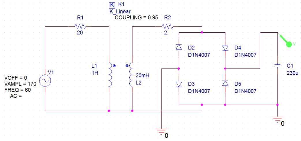
Even though we have eliminated the alternating portion of the current, we still need to maintain the current/voltage level to ensure that the system keeps running. Thus, we connect a capacitor to the circuit to smooth the current. To calculate the minimum capacitance required for the smoothing capacitor to have 1% ripple effect,
