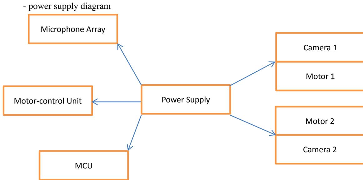
**Figure2 Power supply diagram**
