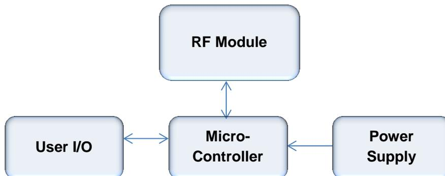
Figure 2. Block Diagram of Controller Unit
