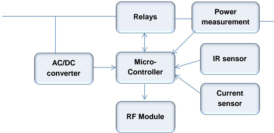
Figure 3. Block Diagram for Sensor Units
