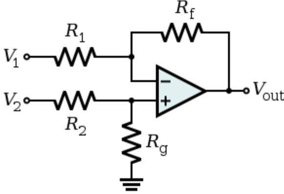
Figure 6.1: differential op-amp circuit
