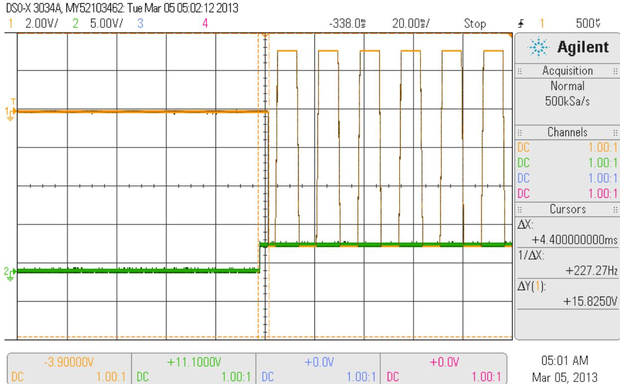
Figure 14.1: Delay between relay switches on operation and control signal
