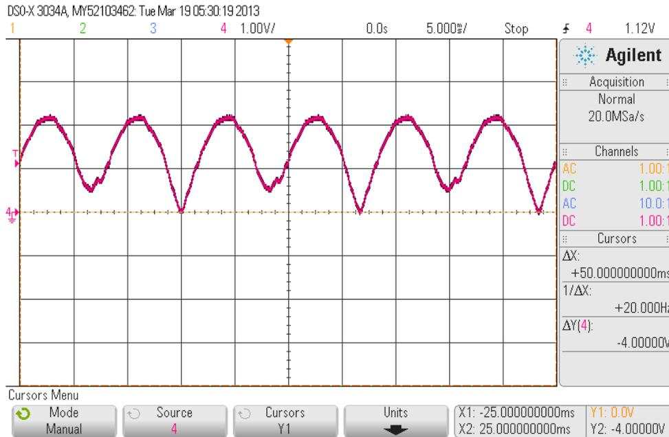
Figure 11.1: After stepped down into 25.7V AC, the Full bridge rectified voltage waveform
