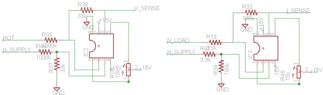
Figure 17.2: The Voltage sensing circuit (Left) and Current sensing circuit (Right)
