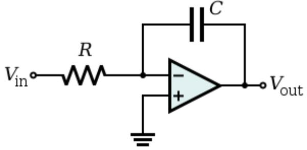
Figure 6.2: integrator op-amp circuit
