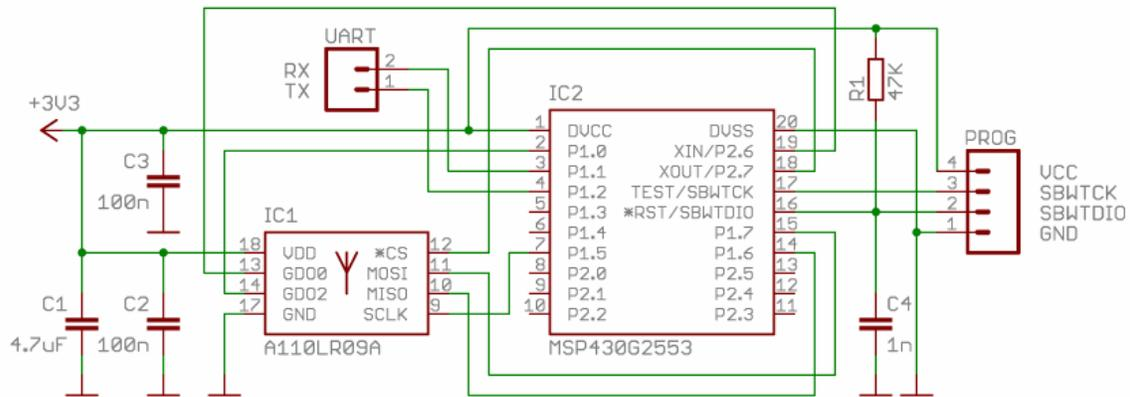
Figure 3: Basic connection of transceiver and microcontroller
