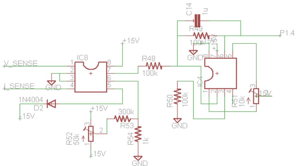
Figure 17.3: Schematic 3.B: The AD633 multiplier circuit (Left) and integrator circuit (Right)
