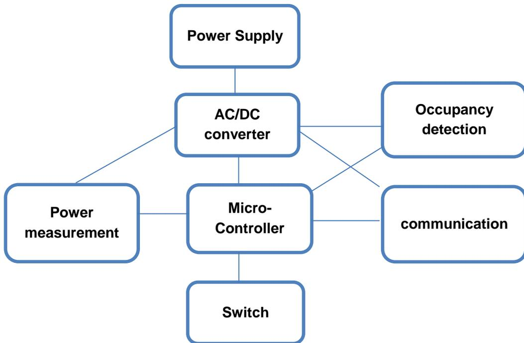
Figure 2.2: Block Diagram for Sensor Units
