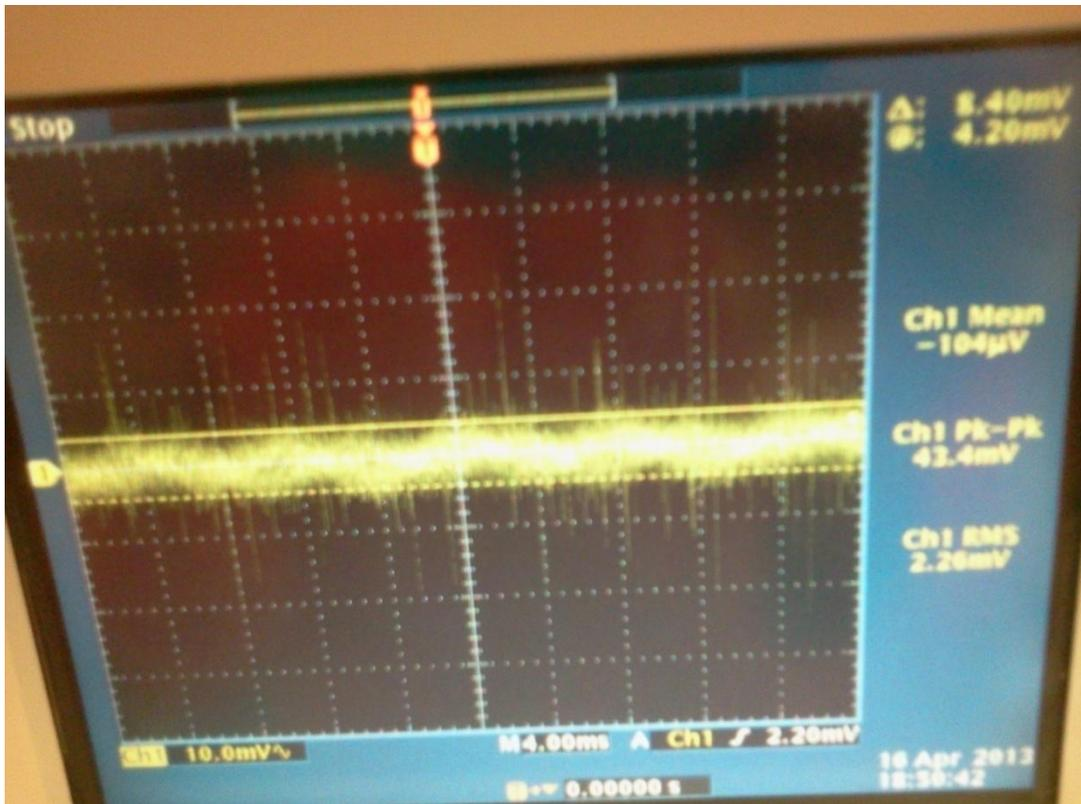
Figure 13: Wither RC filter C=1mF, Ripple is ~8.4mV
