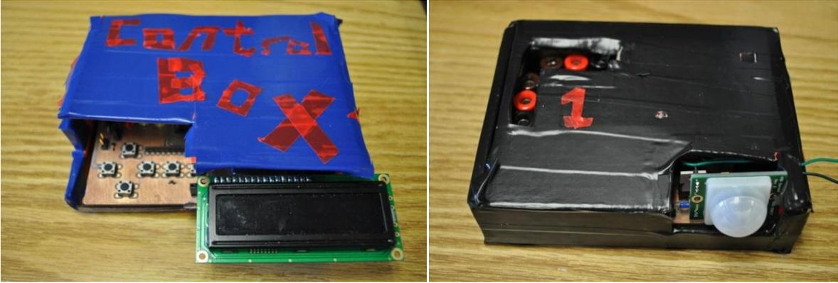
Figure 20: Control Unit's case(Left) and one of the sensor units' case (Right)
