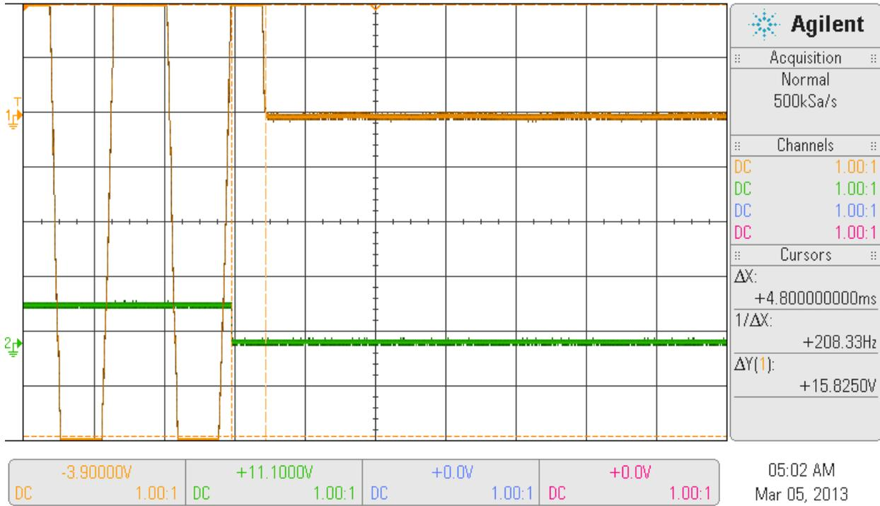
Figure 14.2: a delay between relay switches off operation and control signal
