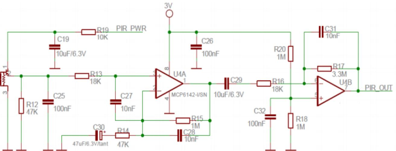
Figure 5: Passive infrared circuit
