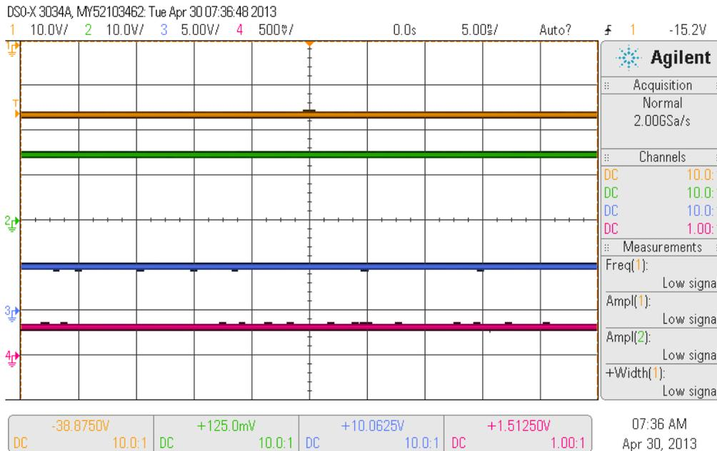
Figure 11.2: The voltage waveform at each voltage regulators output
