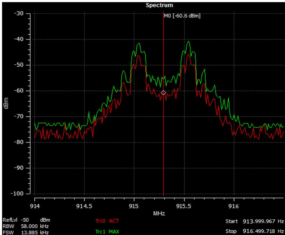
Figure 8.1: Frequency signal at 915MHz operate
