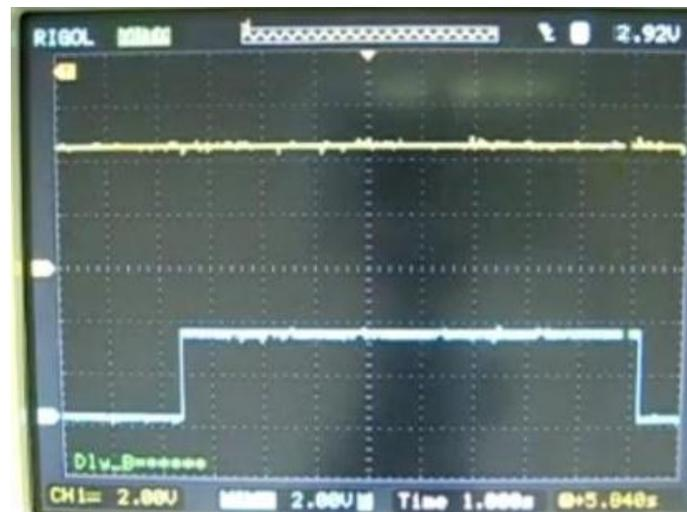
Figure 10: signal from PIR sensor
