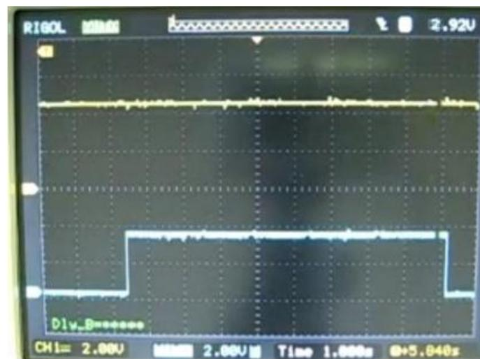
Figure 10: signal from PIR sensor
