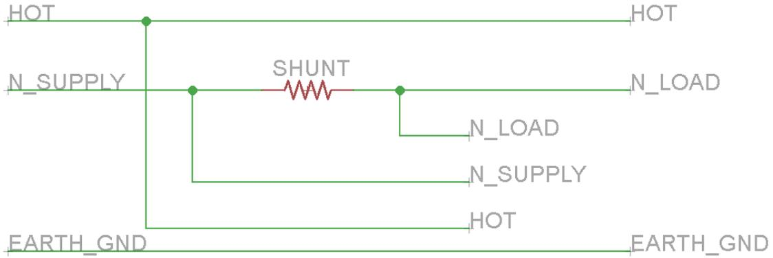
Figure 17.1: The wires for wall power in sensor unit
