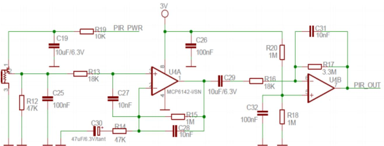
Figure 5: Passive infrared circuit
