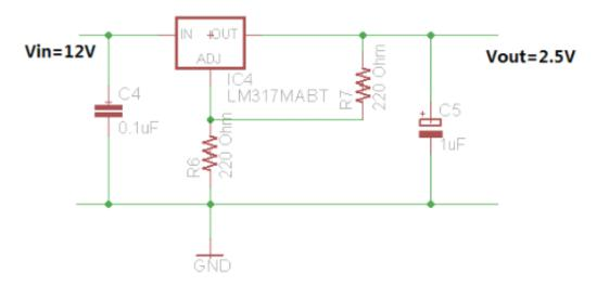
? 2.5V keeps dropping down while connected to the nichrome wire ! Resistance of nichrome wire is too small;
