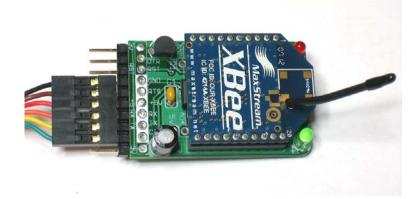
For the receiver XBee, this project will set it up by plugging in the FTDI cable, USB adapter, Arduino, etc. Under windows, check the device manager, look for "USB Serial Port"
