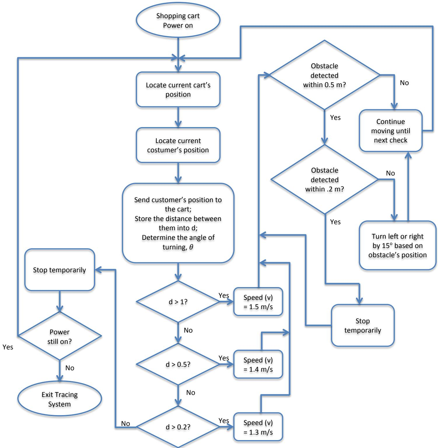
**Figure 7 Tracing system flow chart**
