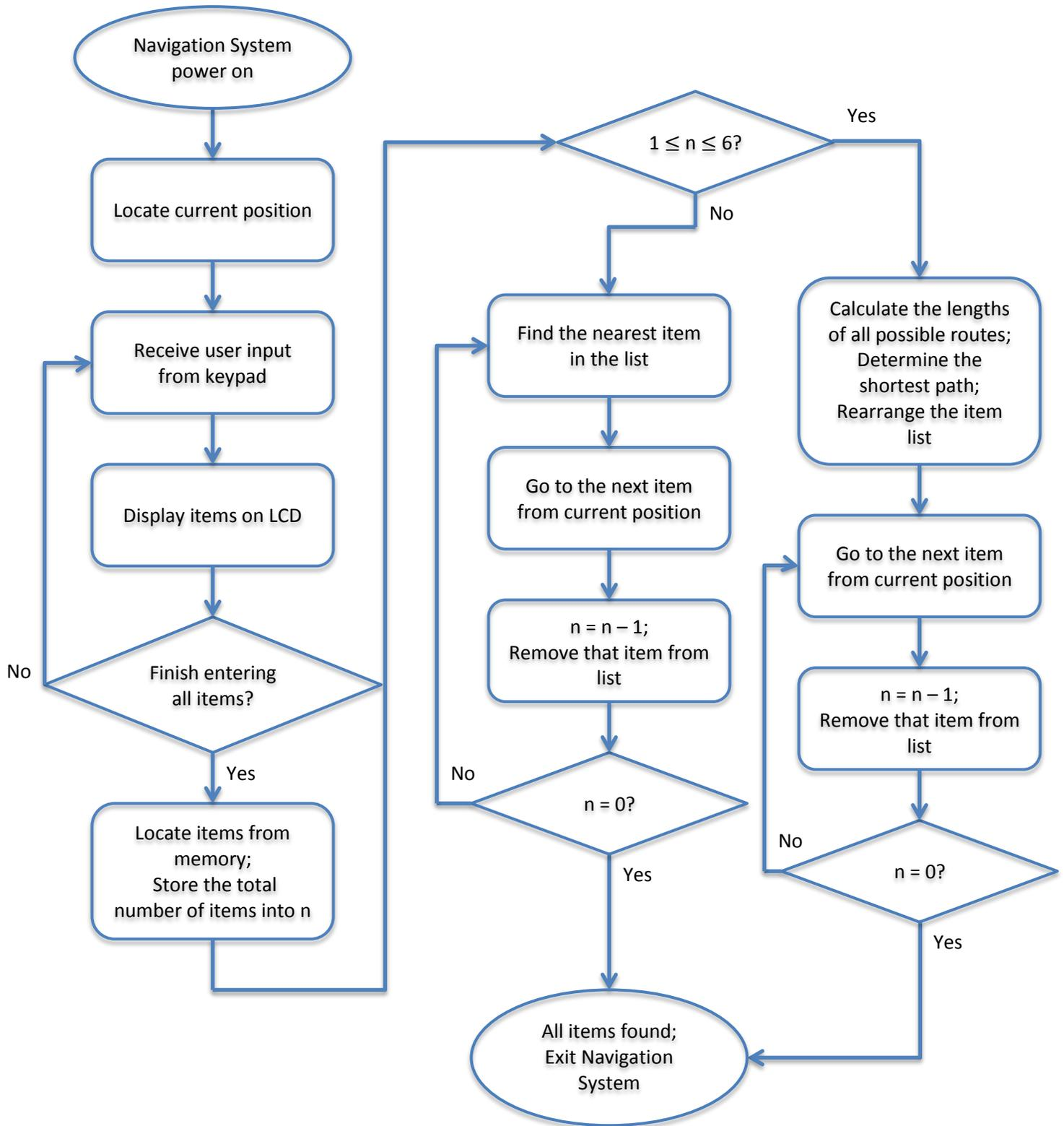
Figure 8 Navigation system flow chart
