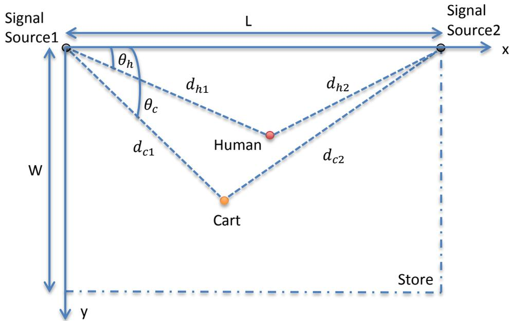
**Figure 2 Position determination process**
