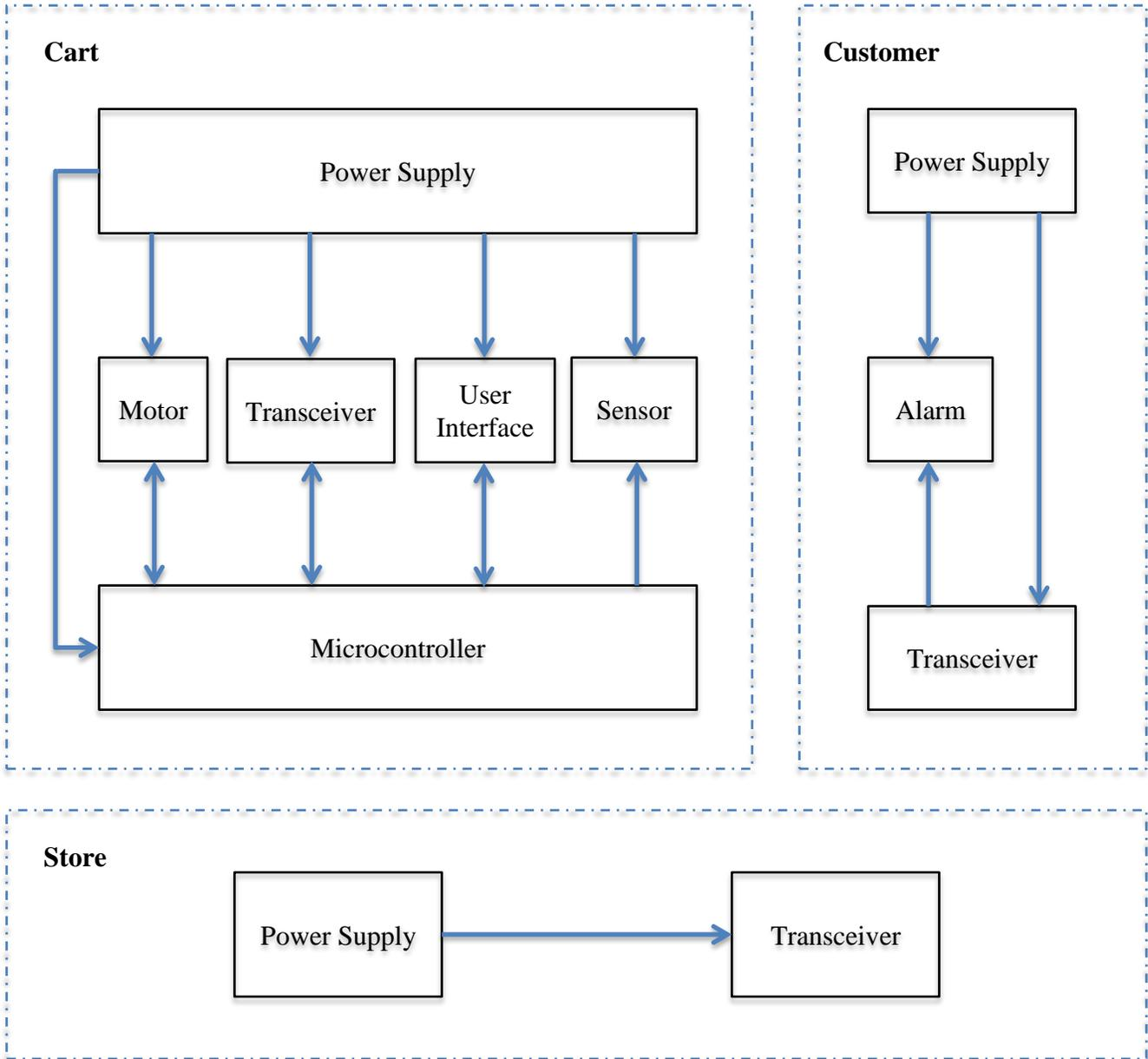
Figure 1 Block diagram
