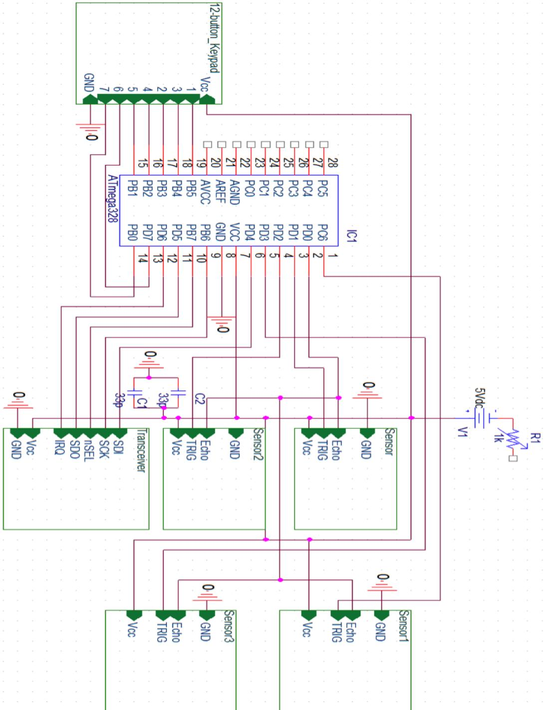
**Figure 4 Schematic for microcontroller, sensors, cart transceiver and keypad**
