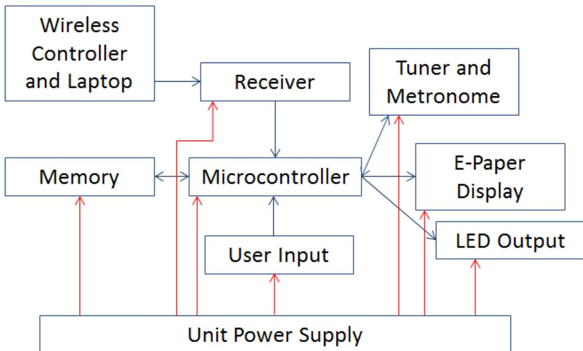
Note: In the diagram, red arrows indicate flow of power, while blue arrows indicate flow of information
