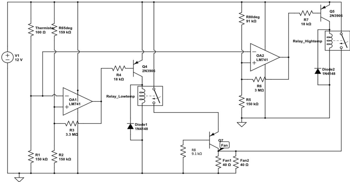
Figure 4: Electrical Schematic for Cooling Controller
