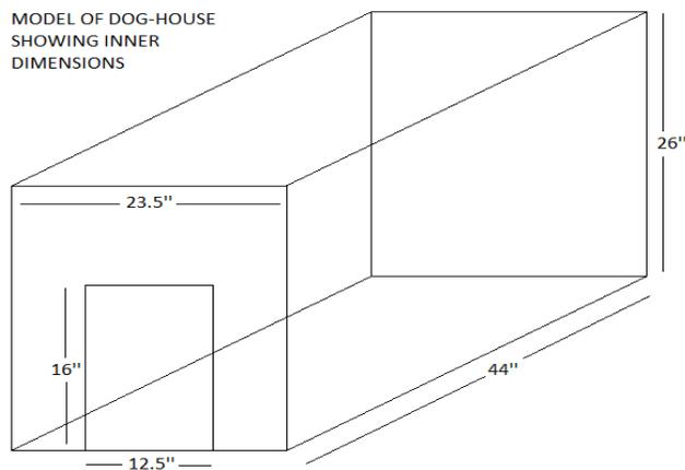
Figure 7: Shows the interior dimensions of the doghouse.
