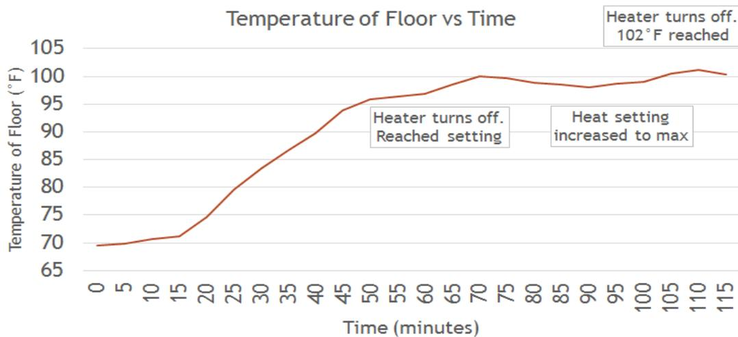
Figure 9: Results of Heating System – Shows the floor temperature increase until user setting is reached. Also shows the emergency temperature shutoff works.
