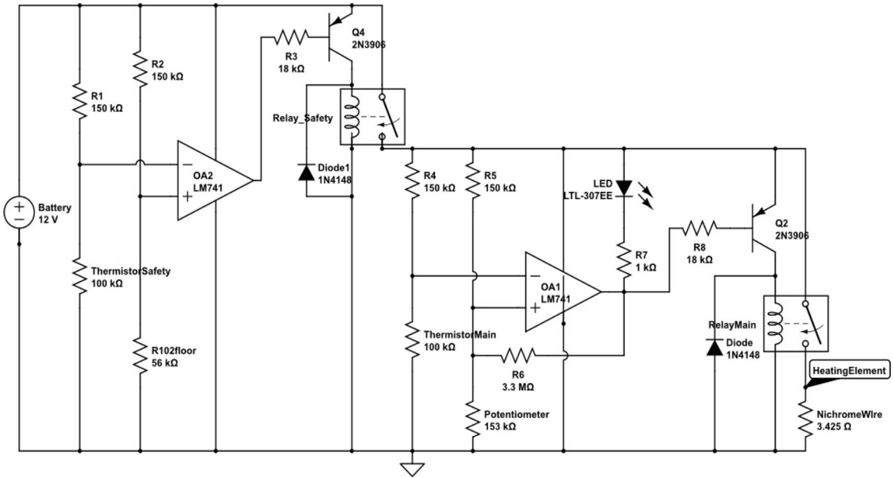
Figure 3: Electrical Schematic for Heat Controller
