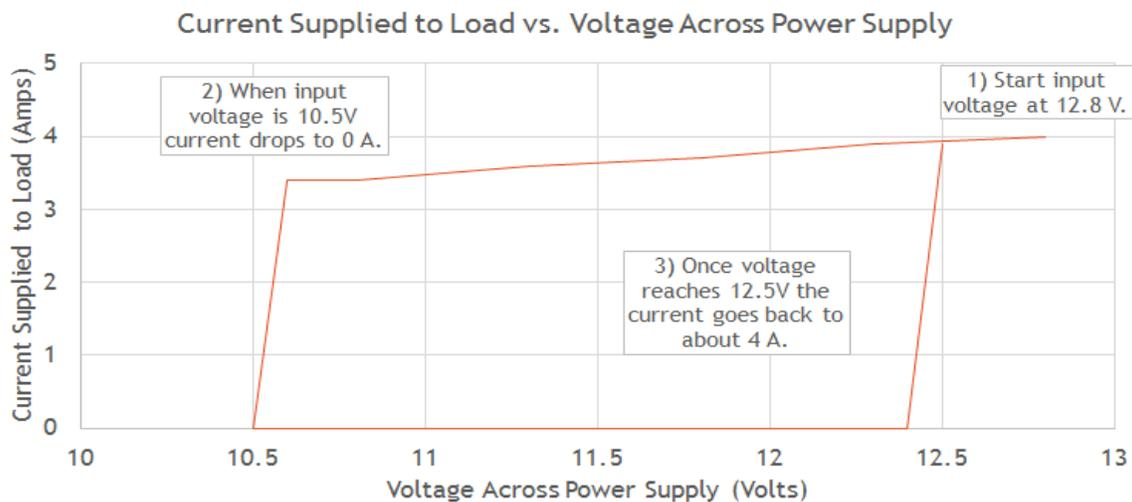
Figure 11: Results of Battery Protection Circuit – Shows the load current being shut off when battery voltage is below 10.5V and then turned back on when the voltage recharges to above 12.5V
