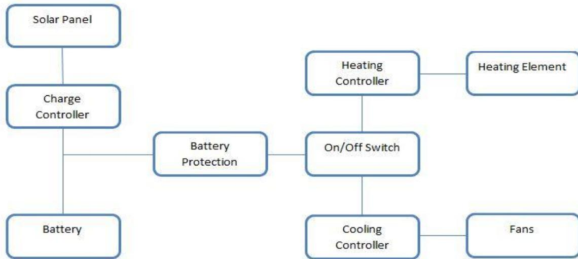
Figure 1: Block Diagram for the Entire Doghouse System
