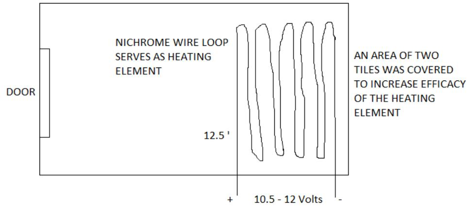
Figure 6: Displays the location of the heating element on floor of the doghouse.
