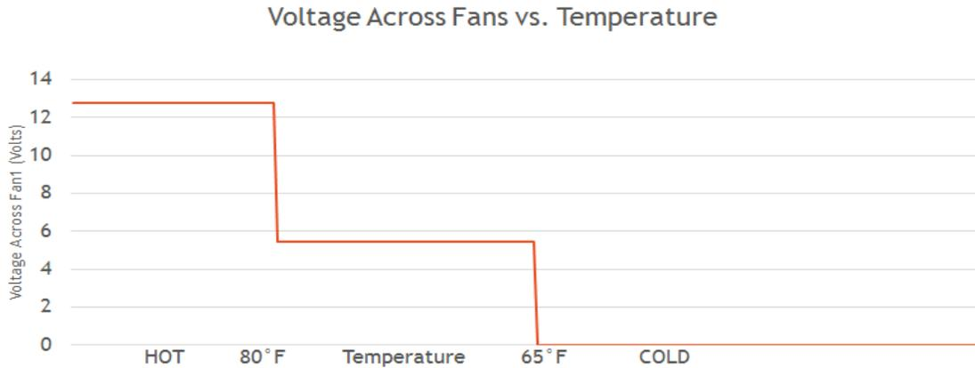
Figure 10: Results of Cooling System- Shows the output voltage of the controller to the fans that correspond to the two speeds, high and low, depending on the house temperature.
