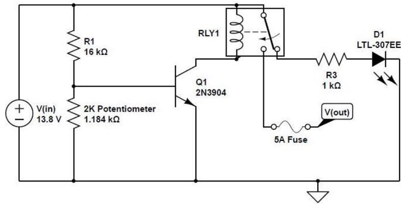
Figure 5: Electrical schematic for the battery protection circuit
