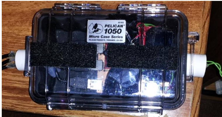
Figure 20: Waterproof Box with PVC Alterations
