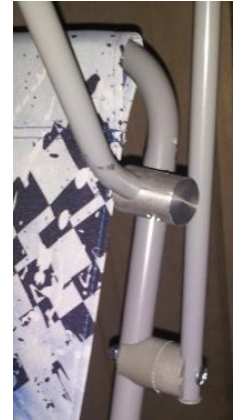
Figure 17: Steel Stopper Added for Canopy Support
