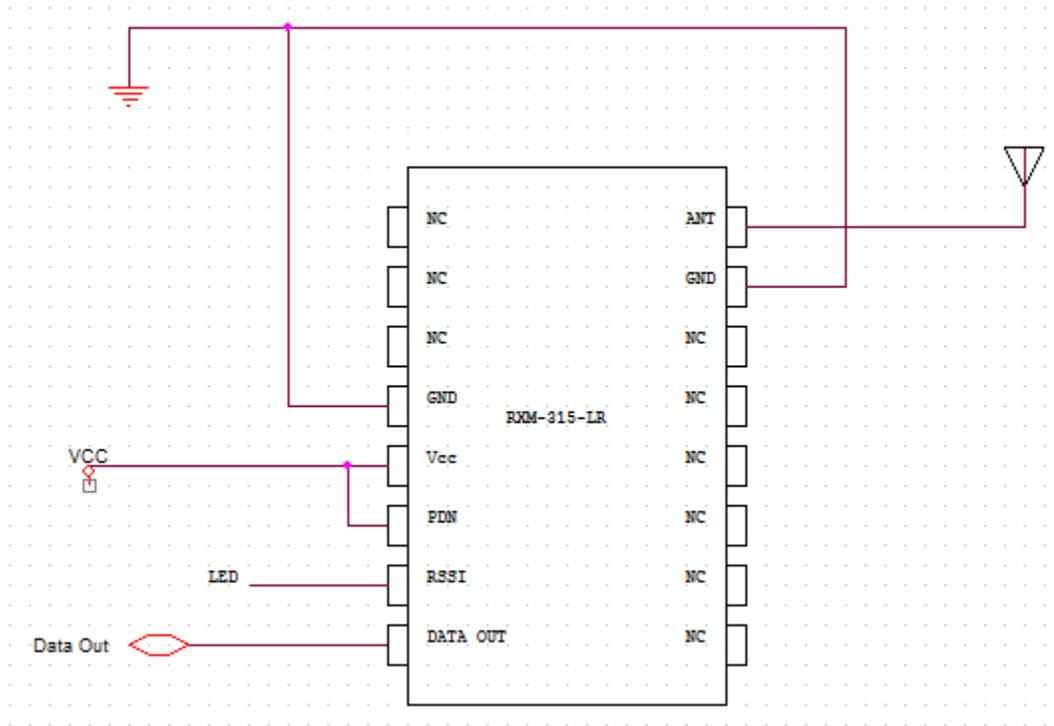
The first stage of the receiver is a band select filter which is fixed at 315 MHz. It picks up the desired signal and filters out the image. The signal is then passed through a low noise amplifier. The amplified signal is down converted to an intermediate frequency by mixing with a local oscillator. The IF signal is then further amplified, demodulated and filtered to recover the original message signal.
