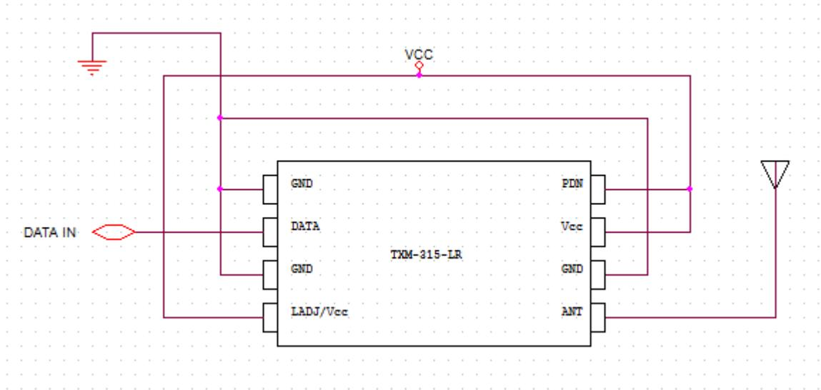
The carrier signal is generated by the built-in VCO which is controlled by a frequency generator. A high precision crystal is used as a reference for the frequency generator. The carrier frequency is fixed at 315 MHz in this case. The carrier signal is then amplified by the power amplifier whose switch is controlled by the DATA input. Therefore, the message signal is digitally modulated and ready to be sent to the antenna after the final filter stage.
