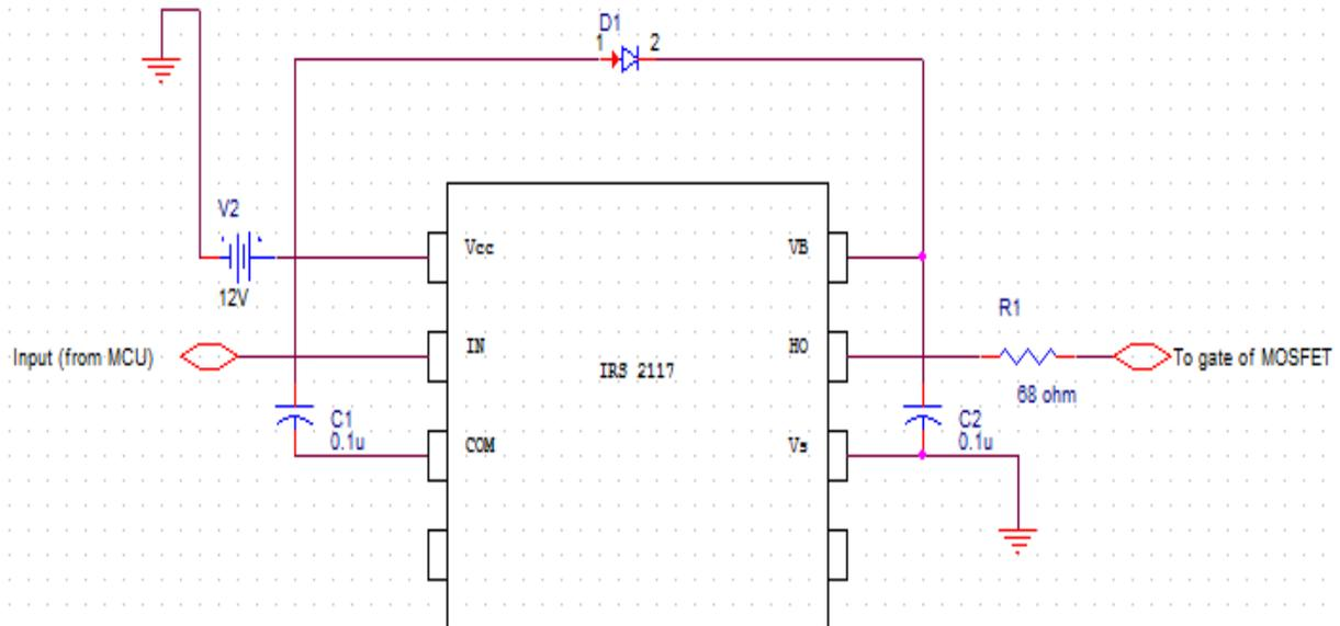
Since it is low side switch control, the source of the MOSFET is connected on the ground. Therefore, the pin V<sub>s</sub> is connected to ground.
