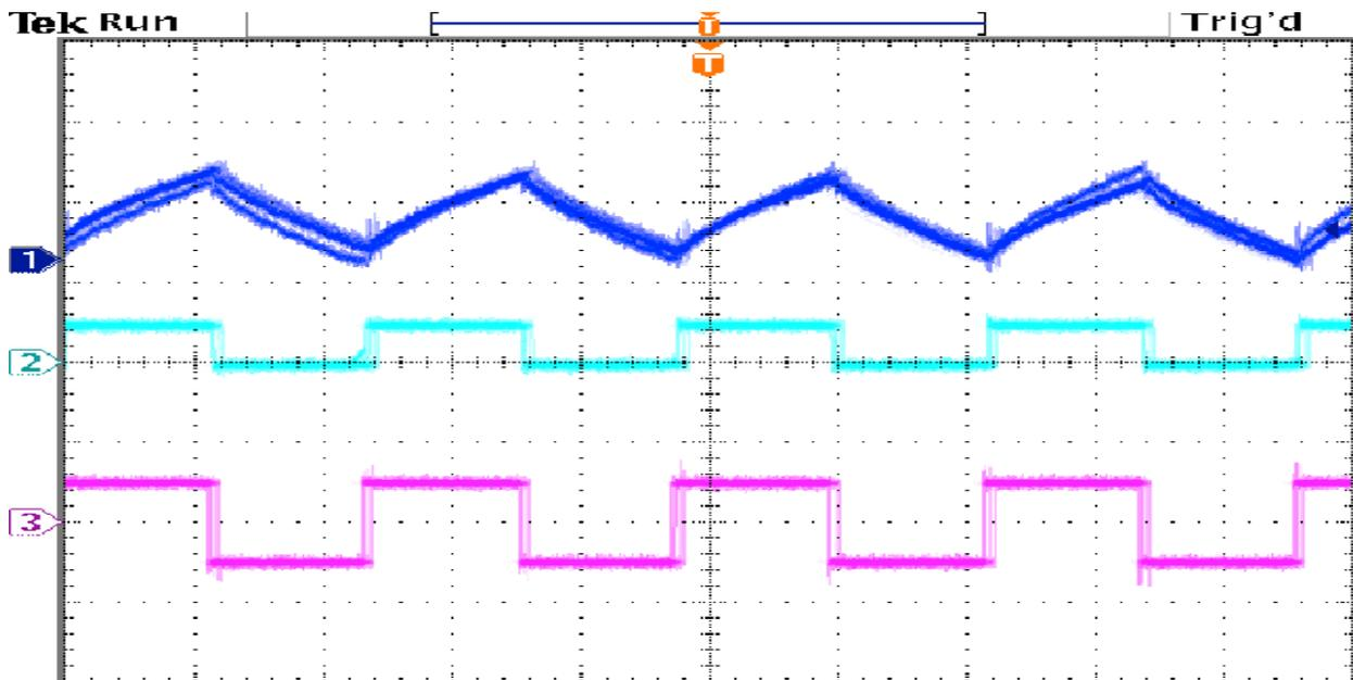
Figure 2. Channel 1: current on the motor; Channel 2: voltage on the motor;
