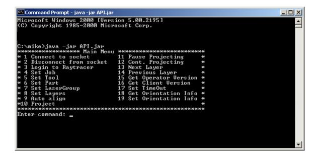
Each of the text commands is sent via a socket to RayTracer Operator. In most cases these commands are the equivalent of pressing the associated controls on Operator's user interface. Thus, sending the "NextLayer" command is equivalent to pressing the "Next Layer" button on the operator screen).
