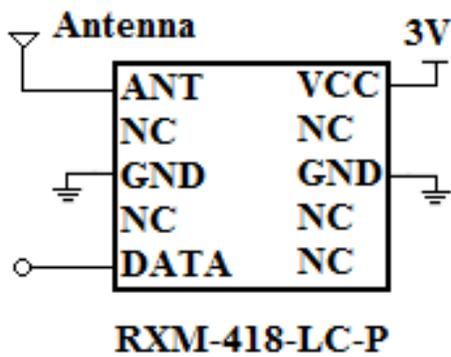
Figure 2. 5 Reciever chip and antenna
