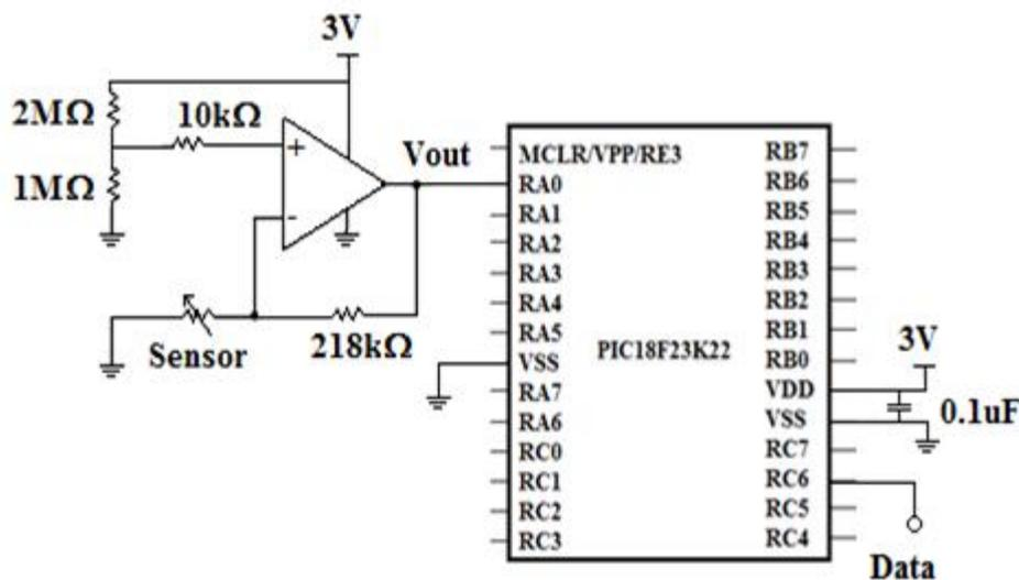
Figure 2. 1 The sensor, non-inverting amplifier and PIC of the sensor module
