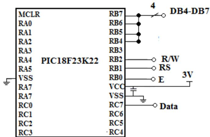
Figure 2. 3 The display module PIC
