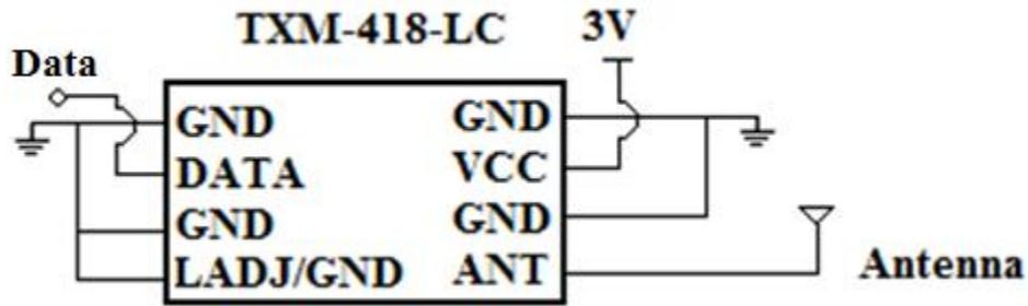
Figure 2. 2 The transmitter and antenna of the sensor module
