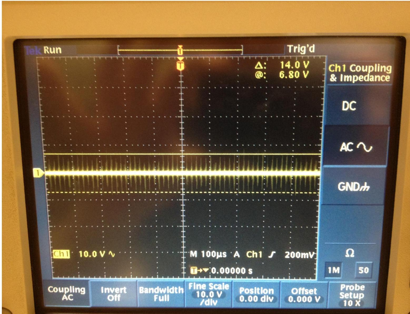
230V ripple measurement = 14Vpp =  $\pm 3.0\%$
