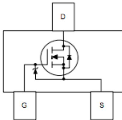
FIGURE 4: Schematic inside FDV301N <sup>[4]</sup>
