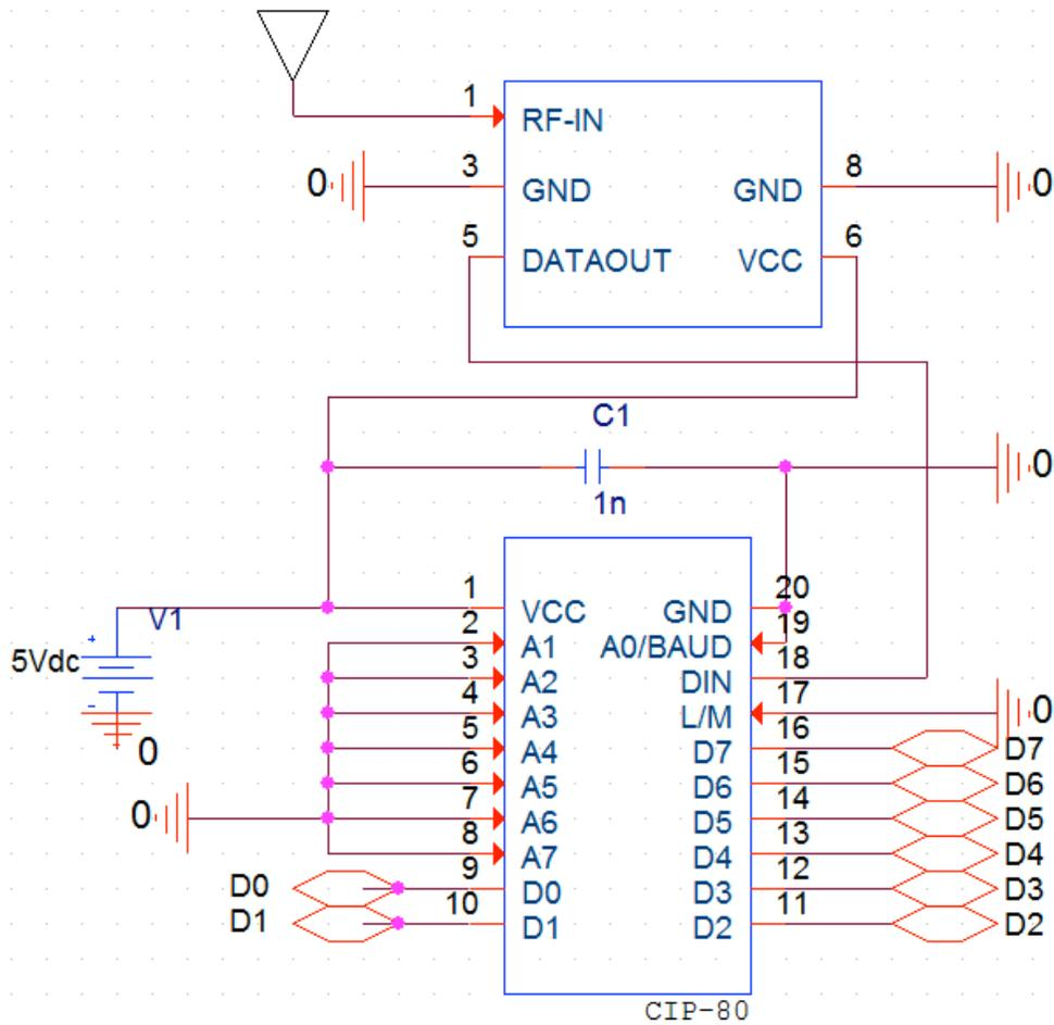
Note: D0....D7 are connected to GPIO of Microcontroller MSP430
