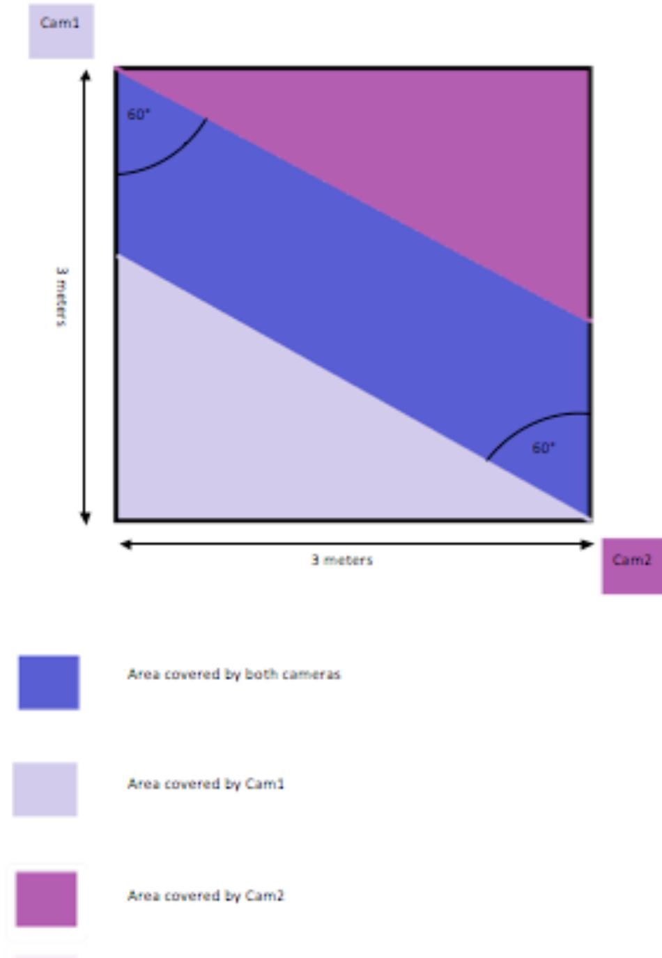
FIGURE 6: Placement and coverage of cameras
