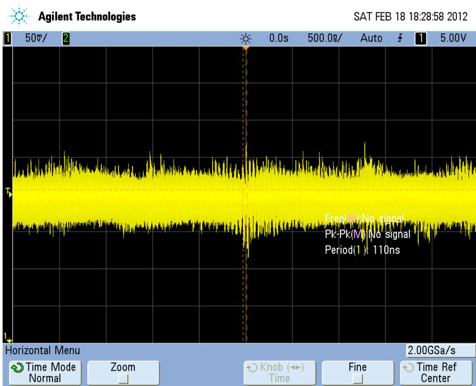
FIGURE 13: 5V DC power supply without 33 $\mu$ F capacitor ( $V_{p-p}$ = 92mV)
