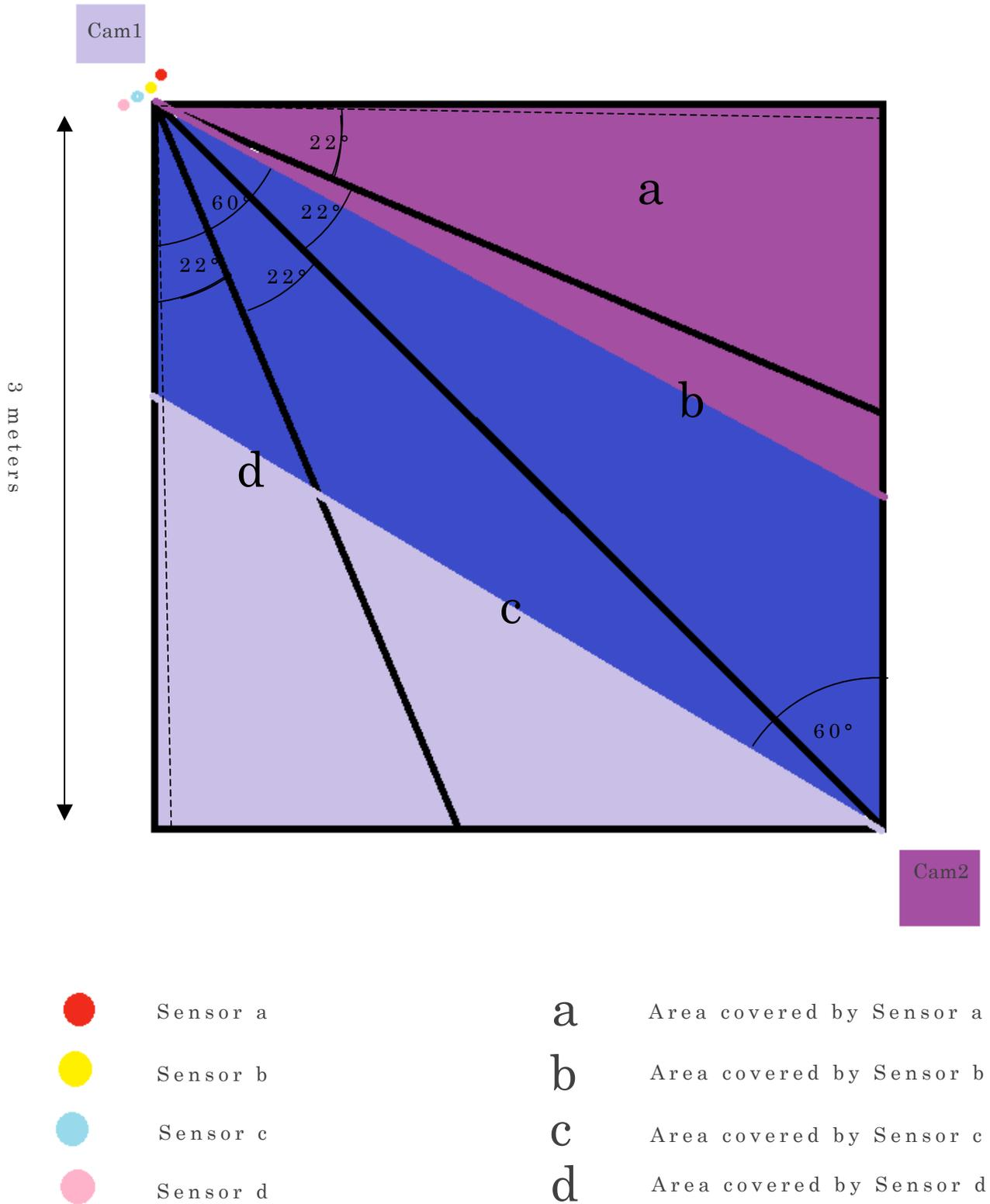
FIGURE 1: Placement and coverage of sensors and cameras
