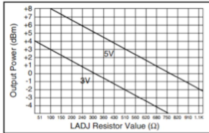
FIGURE 14: Output power vs LADJ Resistor<sup>[9]</sup>
