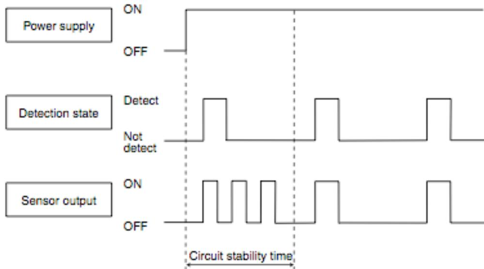
FIGURE 2: Digital output of the sensor (Graph) <sup>[2]</sup>
