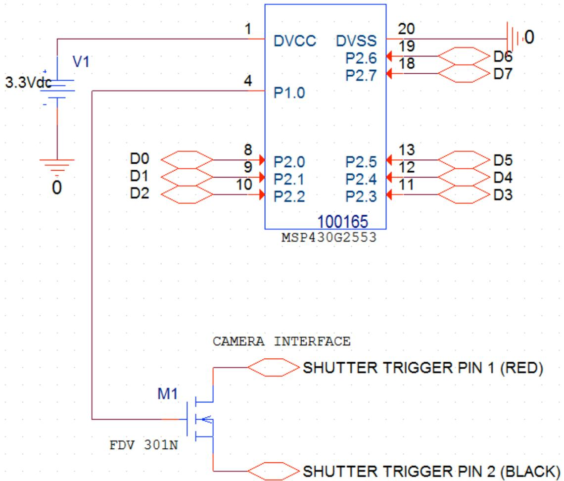
FIGURE 9: Schematic of microcontroller
