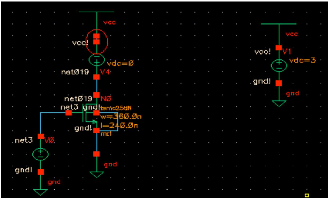
FIGURE 15: Schematic of the simulation of NMOSFET with  $V_{DS}=3V$  and performing a DC Sweep on  $V_G$ .
