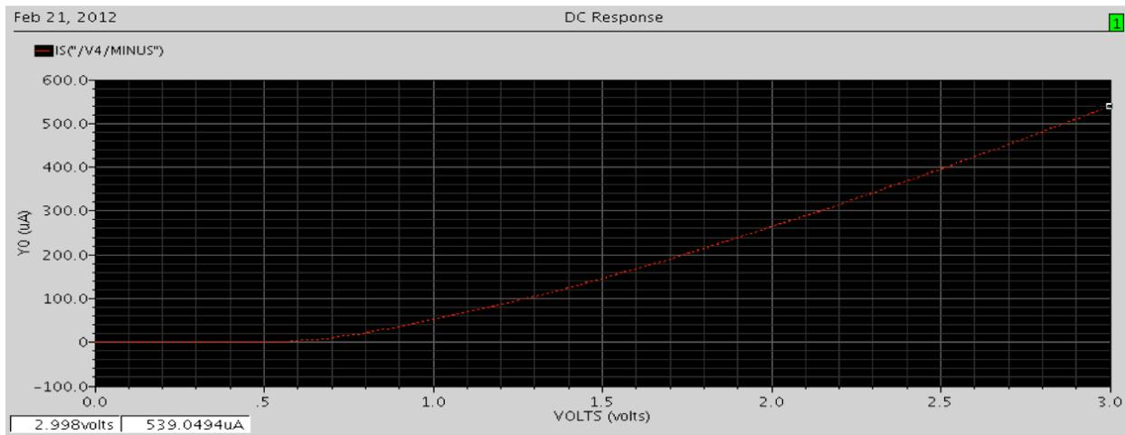
FIGURE 16: Plot of  $I_D$  versus  $V_{GS}$
