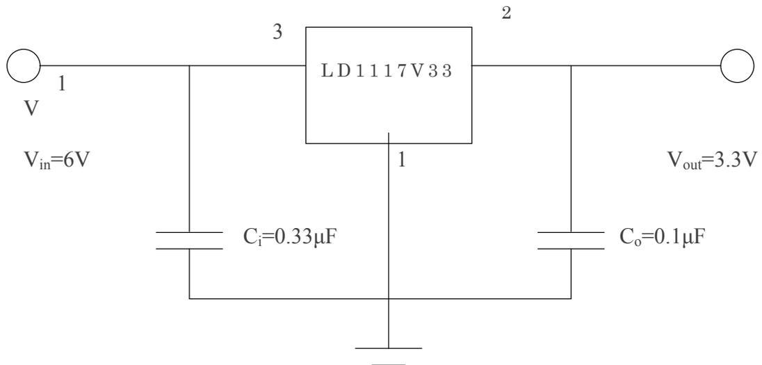
FIGURE 11: Schematic of voltage regulator for Main Controller<sup>[6]</sup>
