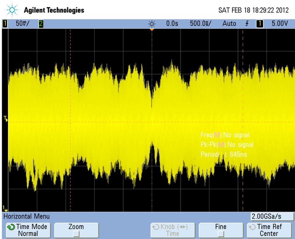
FIGURE 12 : 5V DC power supply without 33 $\mu$ F capacitor ( $V_{p-p}$ = 200mV)
