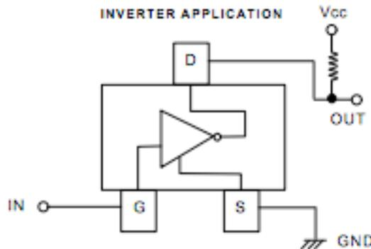
FIGURE 5: Schematic of FDV301N <sup>[4]</sup>
