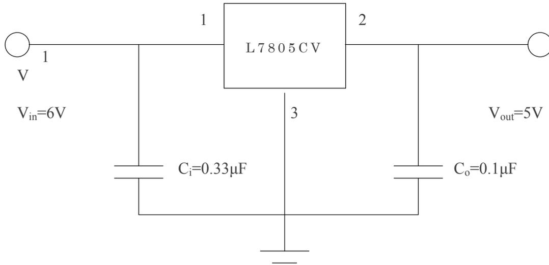
FIGURE 10: Schematic of voltage regulator for Sensing module and Wireless Communication module<sup>[5]</sup>
