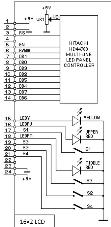
16 × 2 LCD display will display the message that we pre-program in the LCD microcontroller, and interact with user input signal. User can change menu, select mode, and set up time by using the buttons. The buttons are connected with the LCD microcontroller, once it receives the signal, it will change the display on the LCD.
