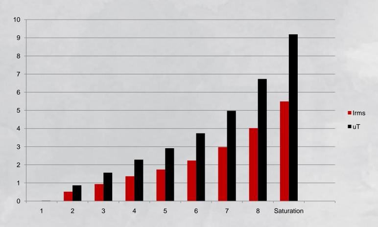
Chart shows input current and corresponding magnetic field levels, and the number of micro-transducers turned on
