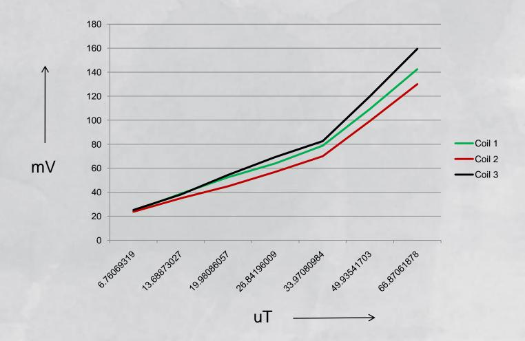
A graph Showing Voltage Induced vs Magnetic Field for each coil separately
