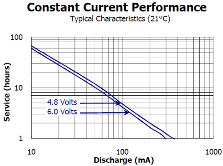
Figure F.1 9V Battery Constant Current Performance
