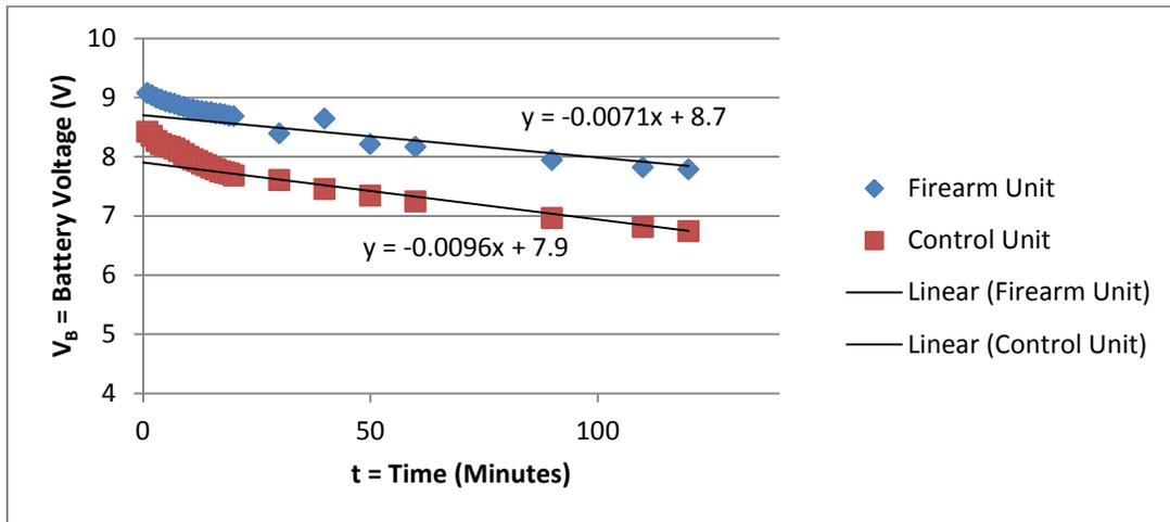
Figure E.1 Voltage vs. Time for Control and Firearm Batteries
