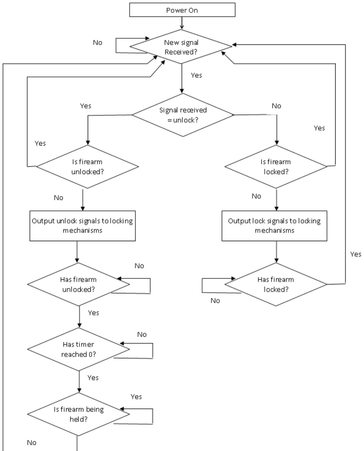
Figure C.2 Firearm Microcontroller Flowchart
