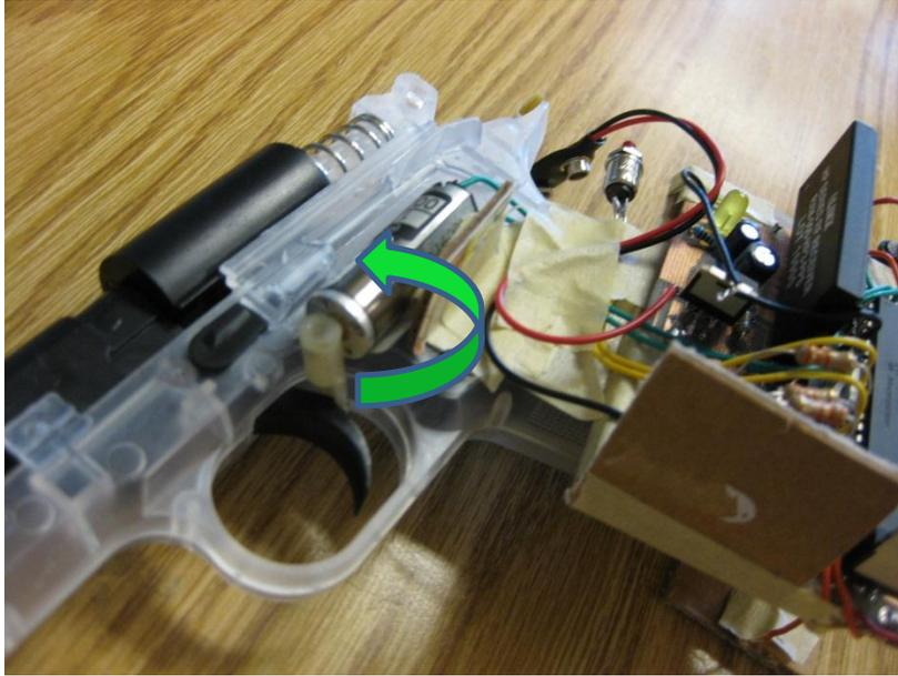
Figure H.5 Trigger Lock
