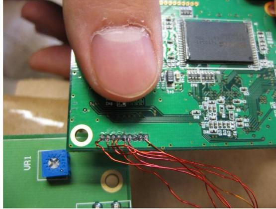
Figure H.1 Fingerprint Scanner Connector Pins
