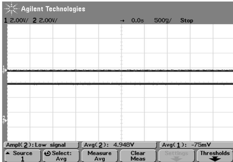
Figure G.3 Pressure Sensor Input & Output – Not Pressed
