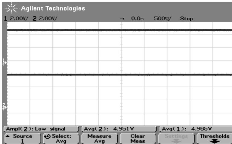
Figure G.4 Pressure Sensor Input & Output –Pressed
