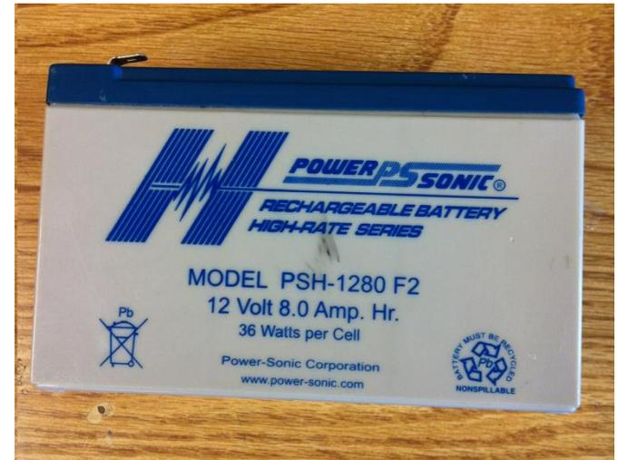
$$\text{Battery Life} = \frac{\text{Capacity}}{\text{Current Draw}} = \frac{8000 \text{ mA Hrs}}{720 \text{ mA}} \approx 11 \text{ Hrs}$$
