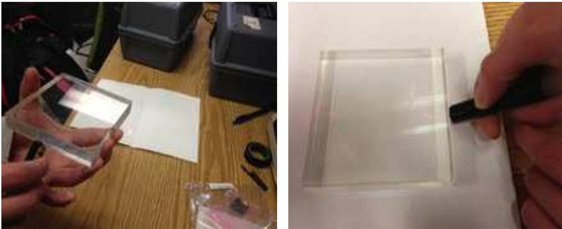
Figure 8: Total internal reflections in an acrylic sheet using a laser light source.
