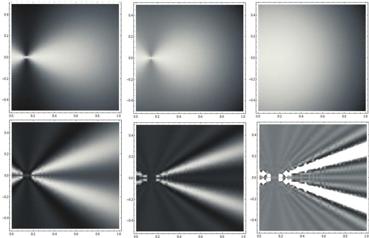
*Figure 15: Directivity of Current Speaker Configuration using Frequencies of 1000(top left), 500(top middle), 80(top right), 5000(bottom left), 10000(bottom middle), 20000(bottom right).*
