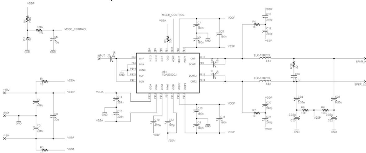
Figure 11: Solid State Power Amplifier Schematic
