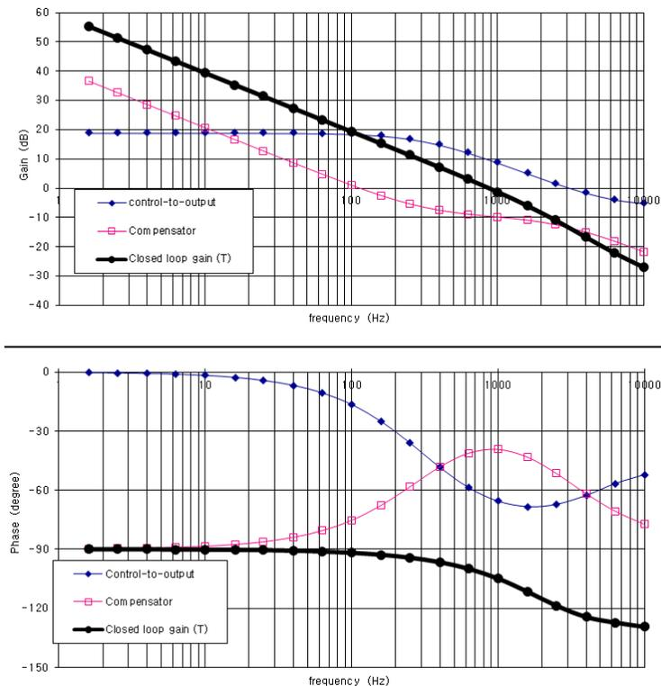
Figure 3: Power Supply Feedback Loop Frequency Response
