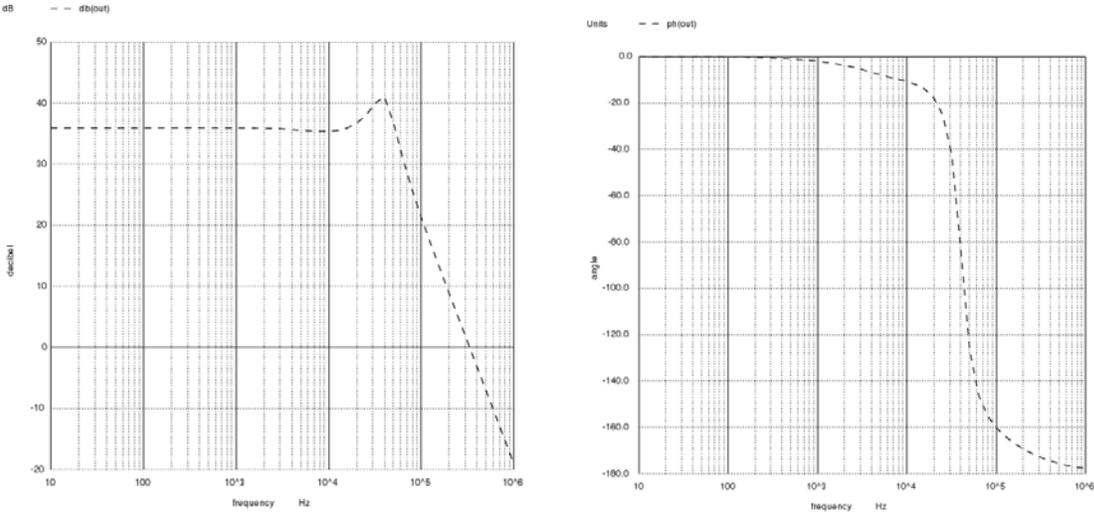
Figure 12: Frequency Response Plots of Loaded Solid State Amplifier
