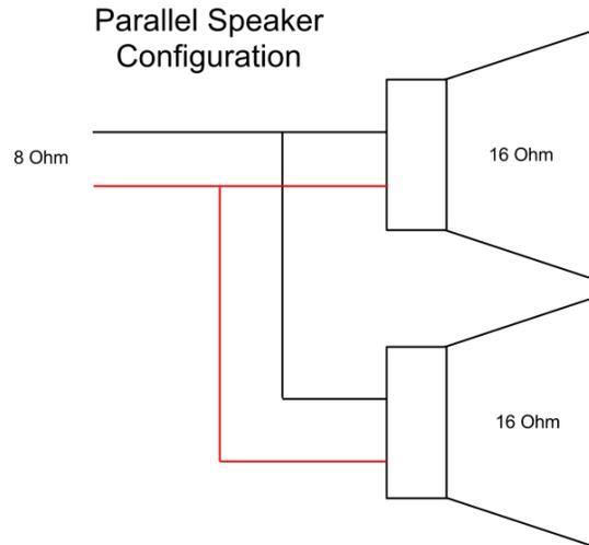
Figure 13: Speaker Wiring Scheme
