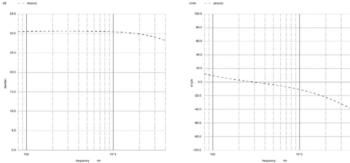
Figure 5: Amplitude (dB) and Phase (°) Simulations of Solid-State Preamp Circuit
