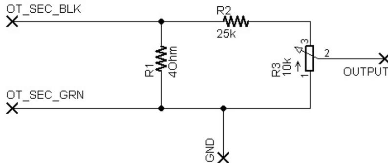
*Figure 9: Resistive Load and Volume Control Schematic*
