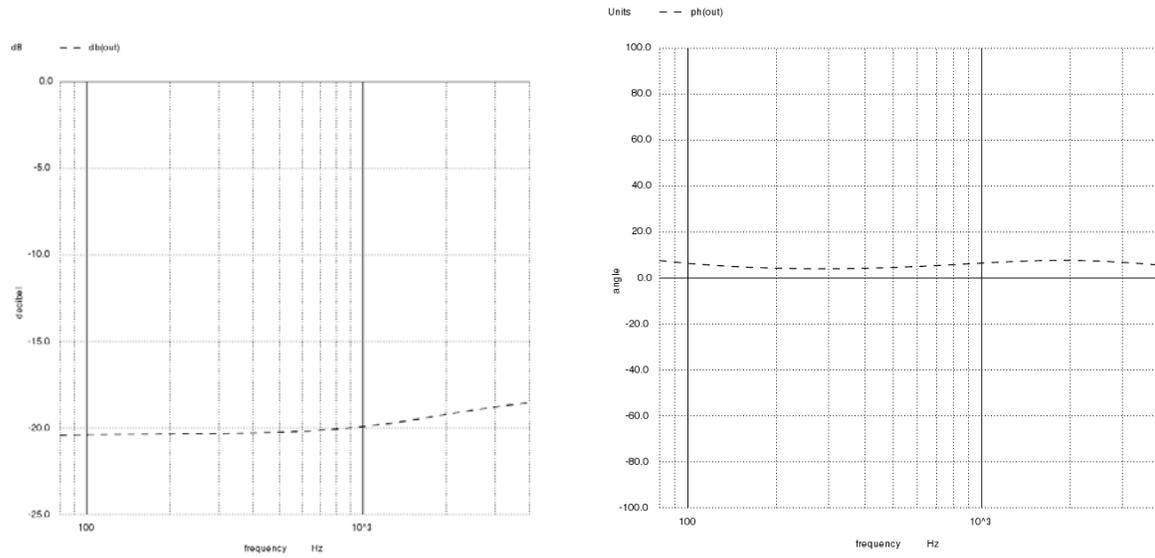
Figure 7: Amplitude (dB) and Phase (°) Simulations of Tone Control Circuit
