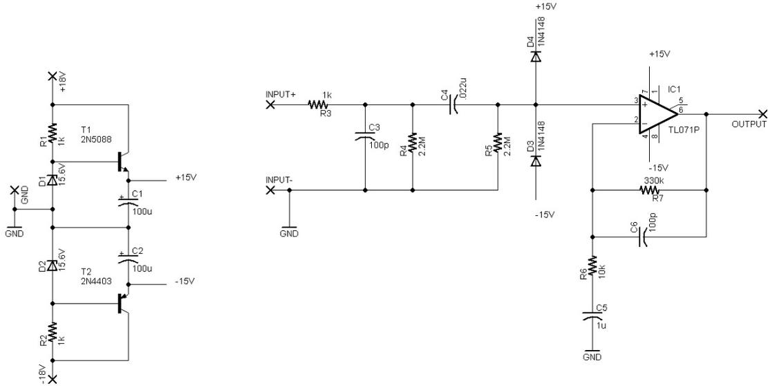
Figure 4: Solid-State Preamp Schematic
