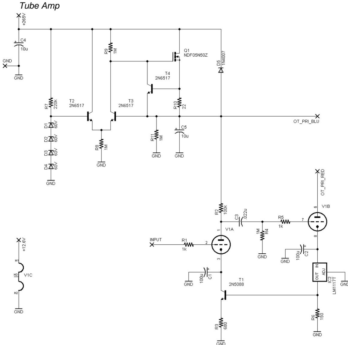
Figure 8: Tube Amplifier Schematic
