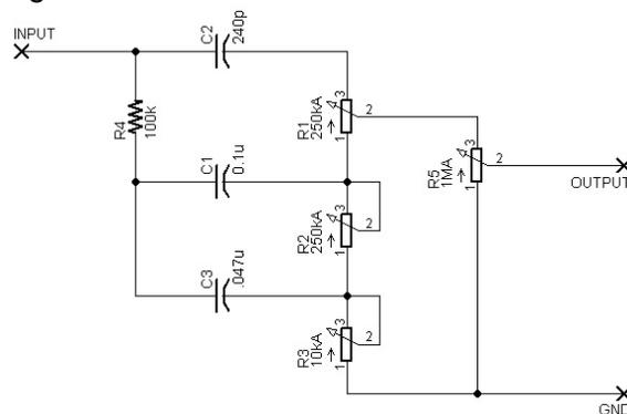
Figure 6: Gain & Tone Control Circuit Schematic
