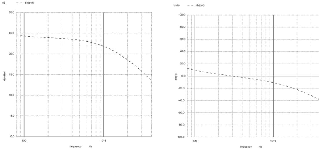
Figure 10: Amplitude (dB) and Phase (°) Simulations of Tube Amplifier Circuit
