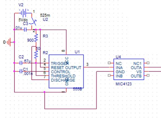
Figure 3. The Oscillating Circuit
