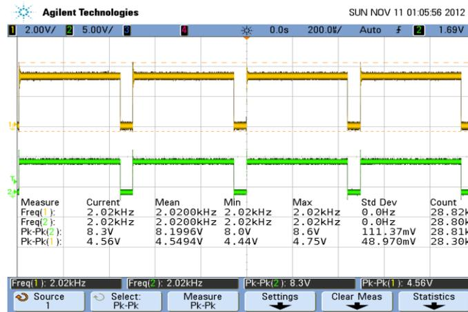
Figure 4. Oscillating Circuit Output
