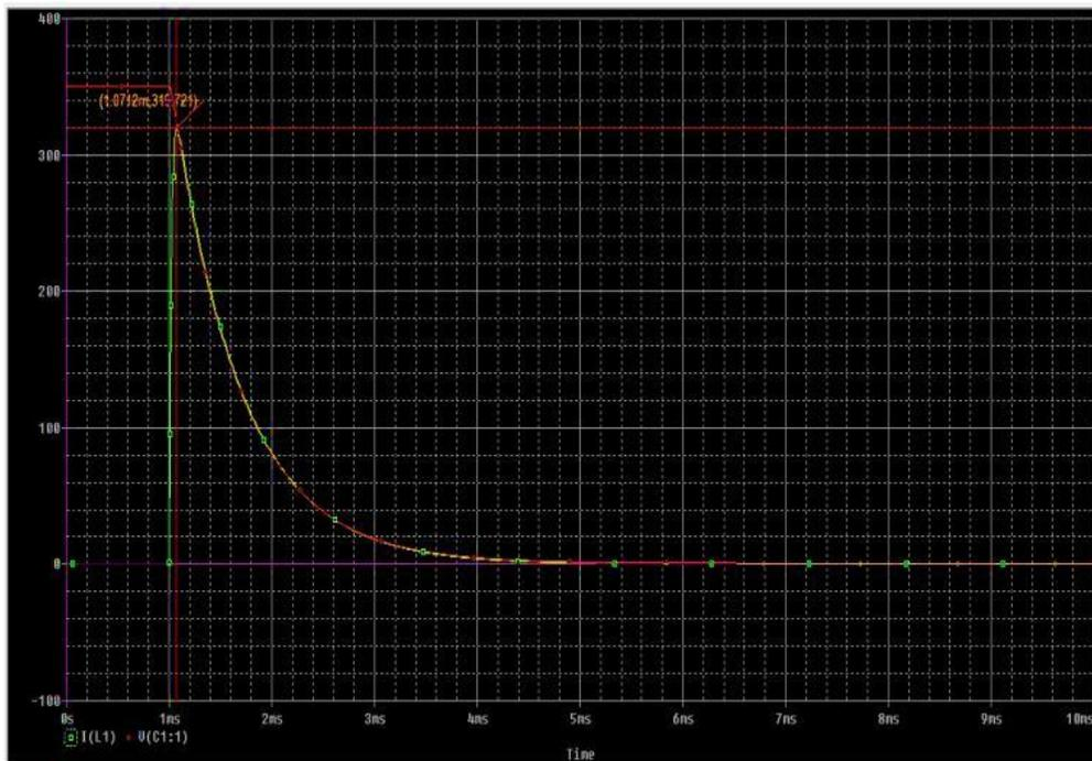
Figure 8. Discharge Curve: The peak current in the coil is 320A
