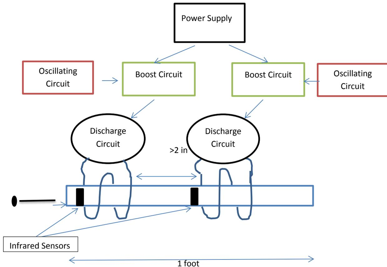
Figure 1. Nail Coil Gun: A connection not shown in this diagram is the SCR from the charging circuit to the inverted output of the infrared sensor.
