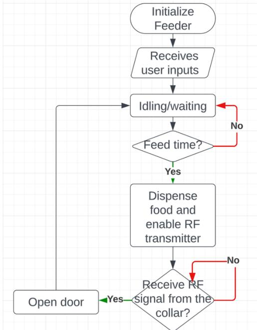
Figure 9 Flowchart of the Programmable Subsystem
