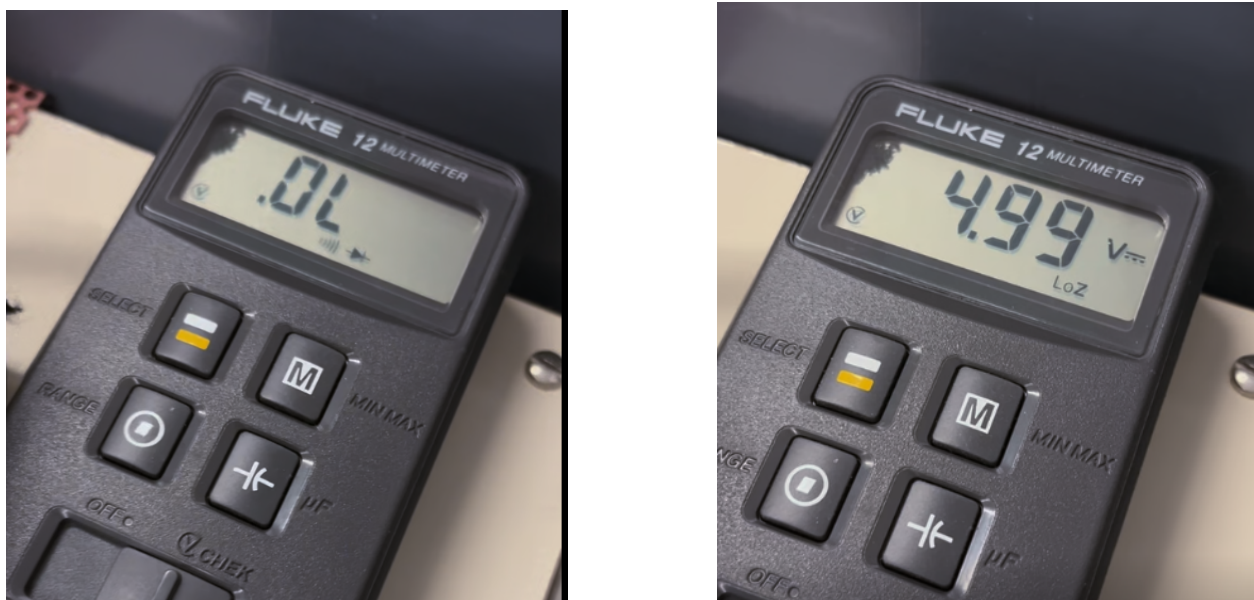
Figure 17: Left: Gate Closed Output Right: Gate Opened Output
