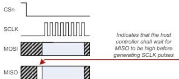
Figure 52 – SPI interface wait state
