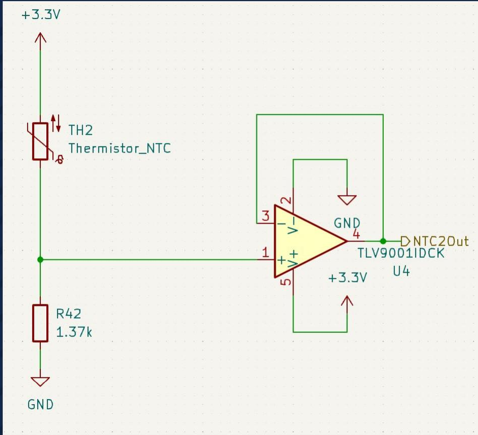
$$R_1 = R_0 e^{\beta(T_1^{-1} - T_0^{-1})}$$
