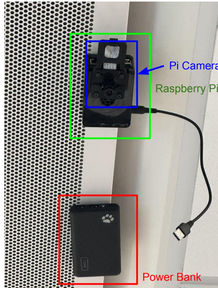
Physical View of the Motion and Object Detection System
