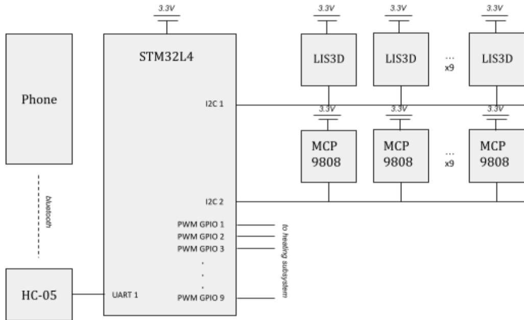
Fig. 3. Control circuit design around our microcontroller.
