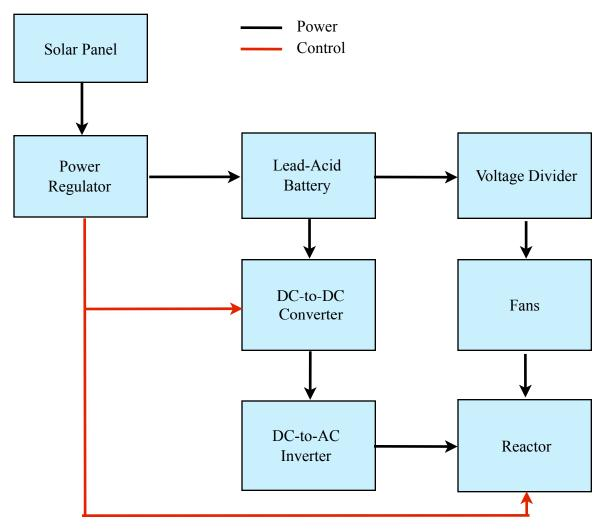
Power Regulator Block Diagram in Detail:
