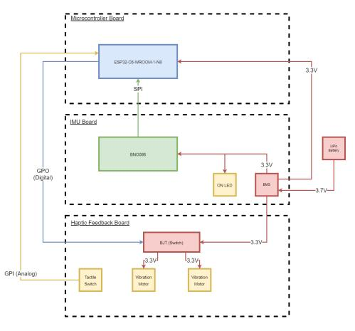
Figure 2: Block Diagram
