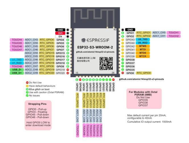
Figure 4: ESP32 Illustrated Pinout [9]
