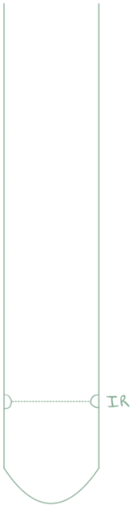
Storage compartment IR sensor interaction
