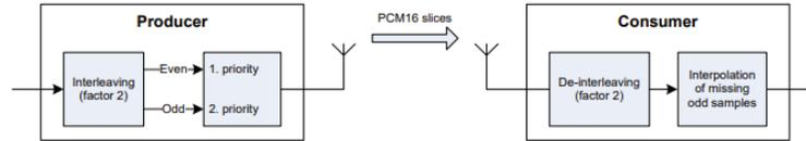
Figure 3: PCM16 Processing Diagram
