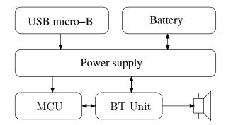
Figure 3: Speaker adapter block diagram
