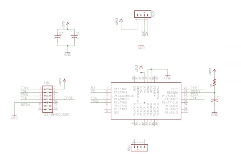
Figure 4: MCU Schematic
