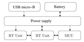
Figure 2: Hub block diagram
