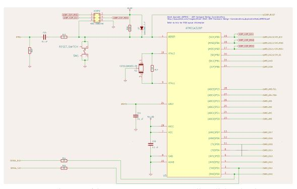
Fig. 8 Zoom-in schematic of the ATMEGA328P microcontroller. All the related components connected in standard configuration according to its datasheet [1].
