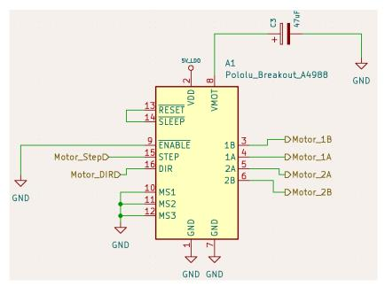
Fig. 9 Schematic of the A4988 motor driver.
