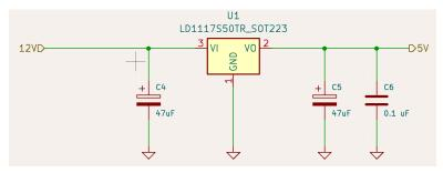
Fig. 6 Schematic for the regulator, receiving 12V from the power supply and providing an output of 5V.
