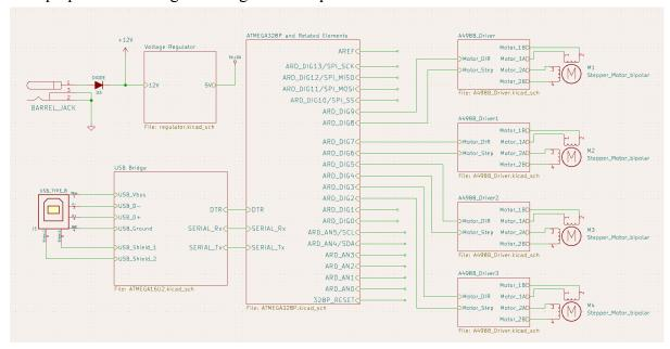
Fig. 5 High level schematic of the circuit subsystem.
