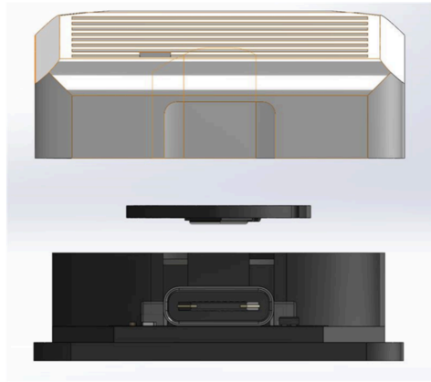
Figure 3: Posterior view of the device, highlighting the USB port and microphone module
