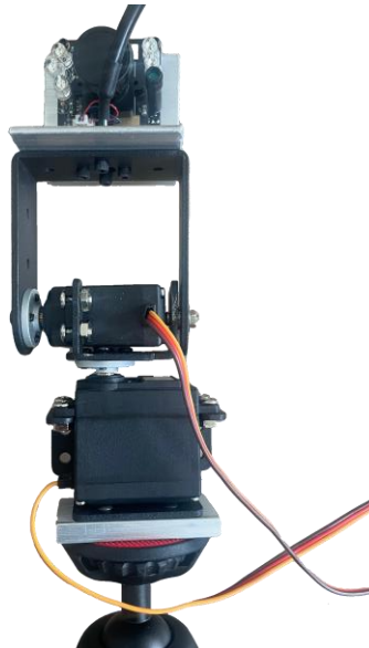
Figure 12: Gimbal Submodule, with the two servo motors as well as the camera submodule
