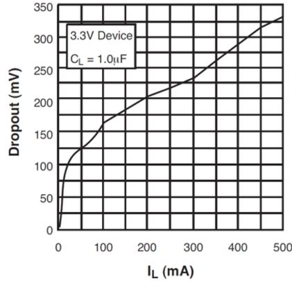
Figure 3: Dropout voltage of the Voltage Regulator
