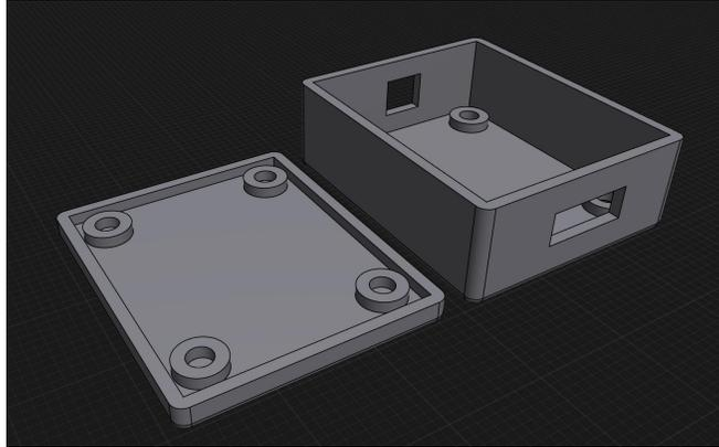
Figure 11: Charger Circuit Enclosure
