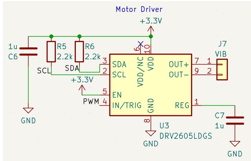
Figure 6: Vibration Subsystem
