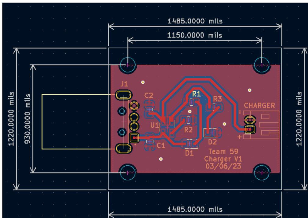
Figure 19: Charger circuit PCB with dimensions
