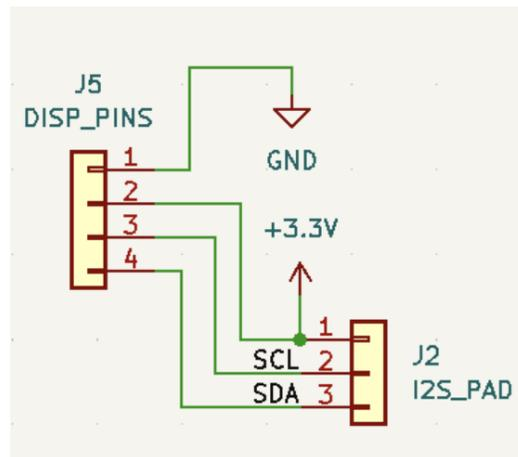
Figure 7: Display Subsystem
