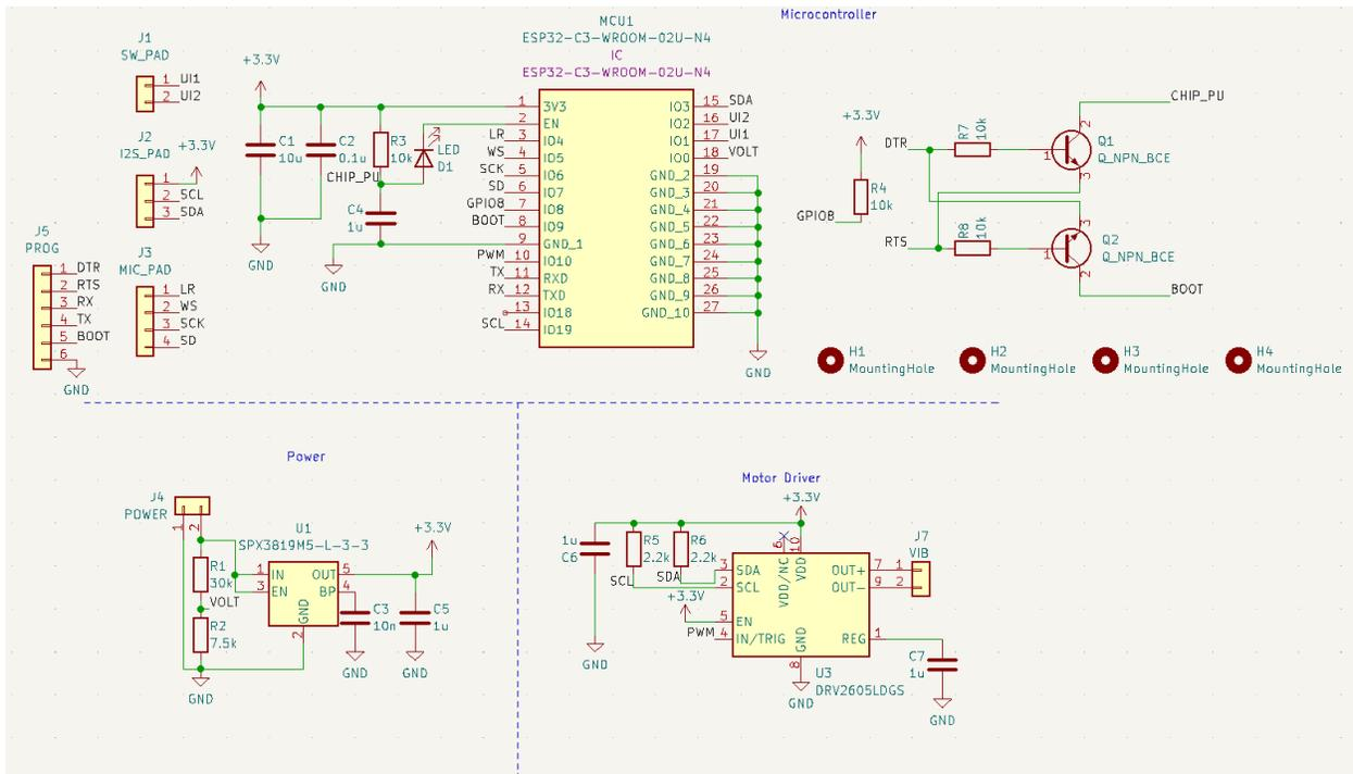
Figure 15: Bottom PCB Schematic
