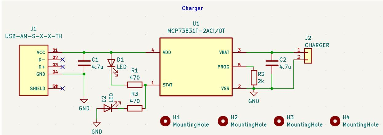
Figure 16: Charger circuit Schematic
