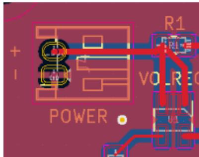
Figure 2: JST connector in bottom PCB
