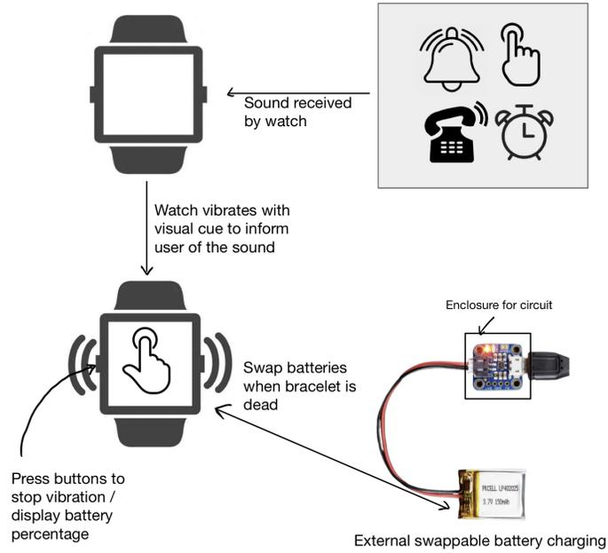
Figure 9: Visual Aid on how the bracelet works
