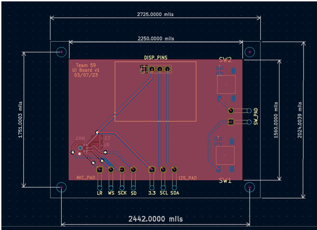
Figure 17: Top PCB with dimensions
