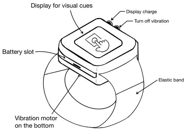
Figure 10: Initial Bracelet Prototype Physical Design
