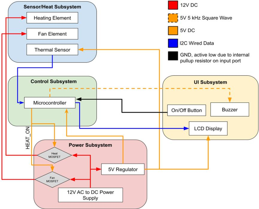
Figure 3: Block Diagram illustrating our final design subsystems and their connections.
