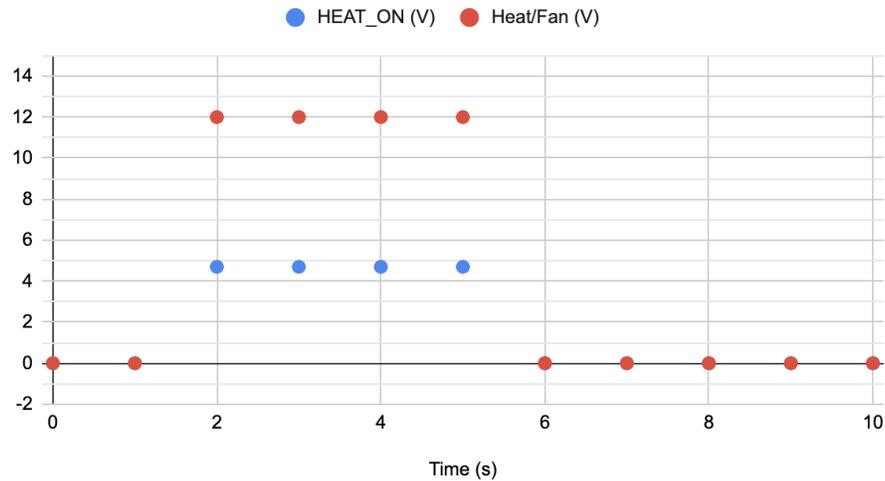
Figure 13: Data Plot of HEAT\_ON Signal and Heat/Fan voltage over time
