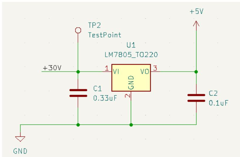
Figure 11: 5V Linear Voltage Regulator
