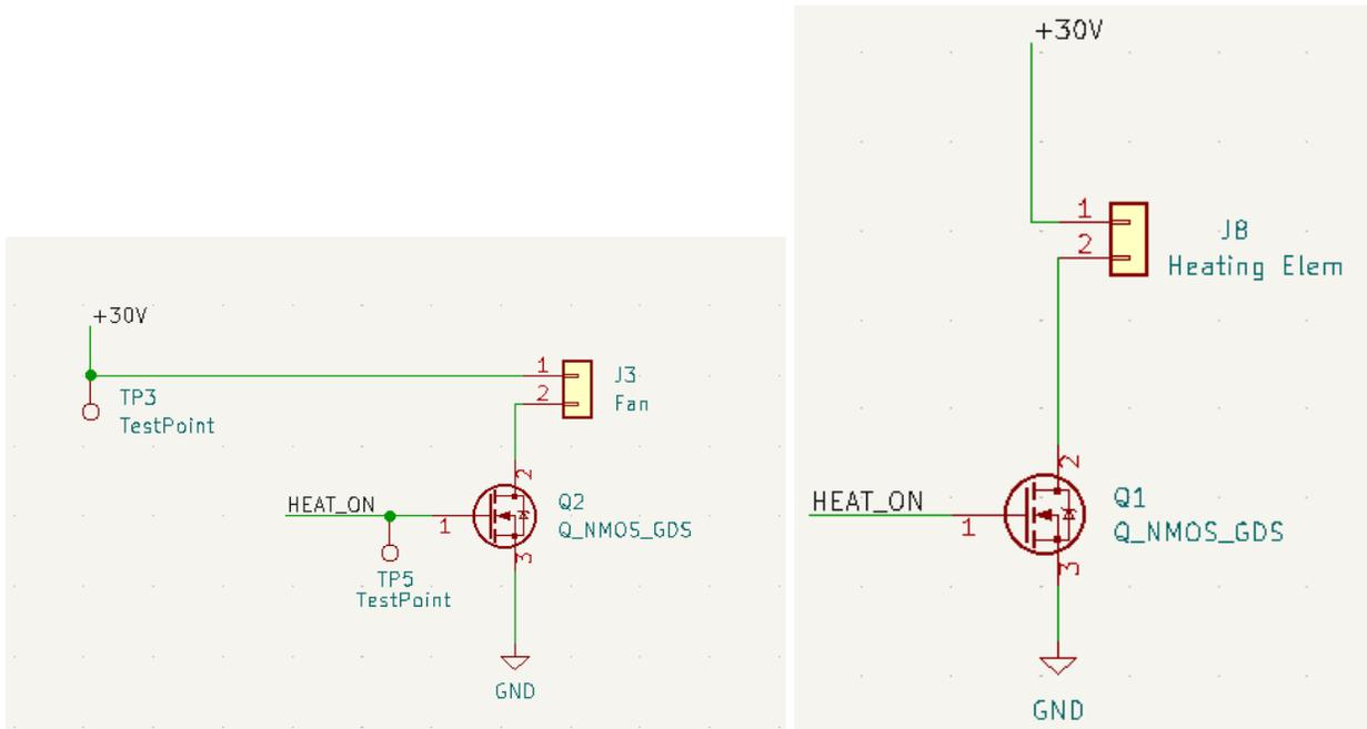
Figure 10: Dual MOSFET wiring from heat subsystem to ground
