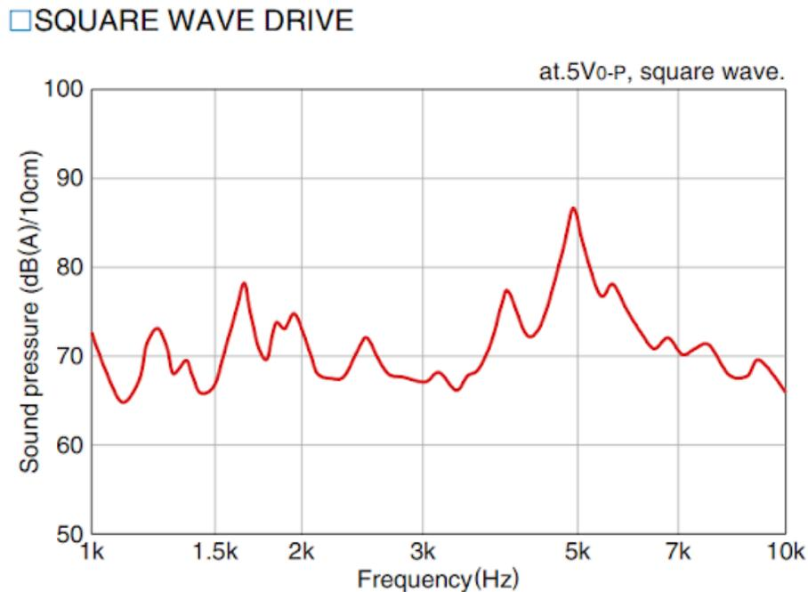
Figure 9: PS1420P02CT Buzzer Frequency Sound Pressure Characteristics.
