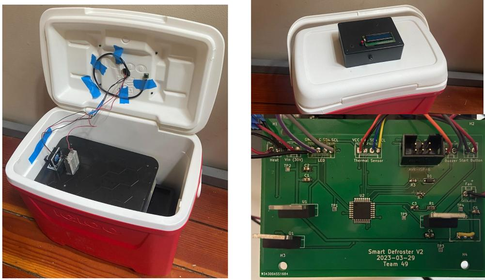
Figure 2: Photos of completed device, internal, external and PCB which is enclosed in the top mounted Polycase.
