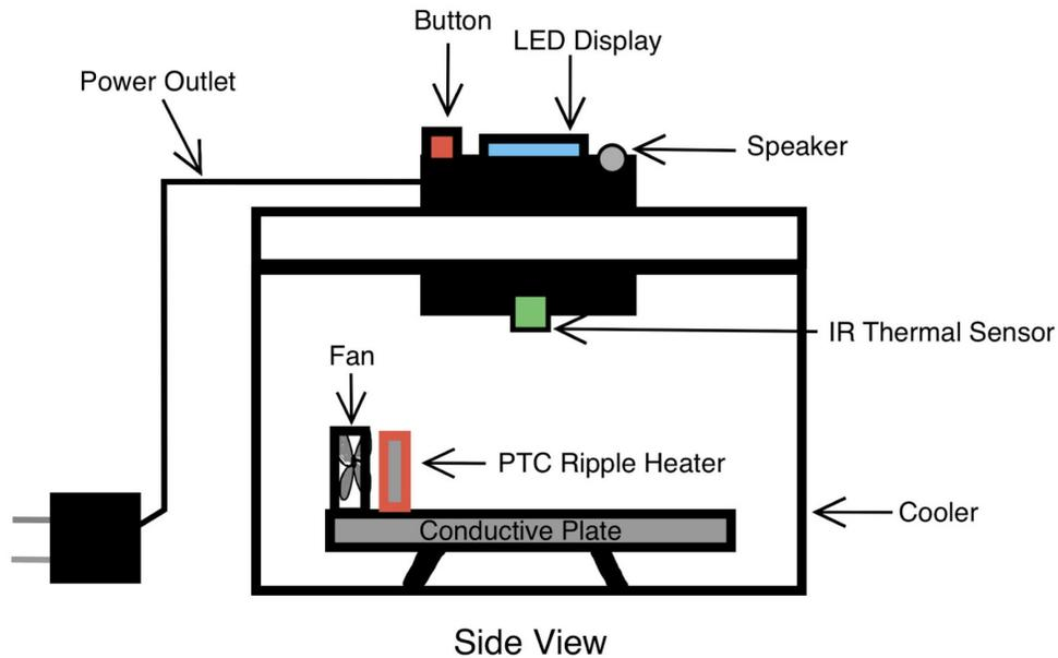
Figure 1: Drawn Diagram of the Meat Defrosting Device.
