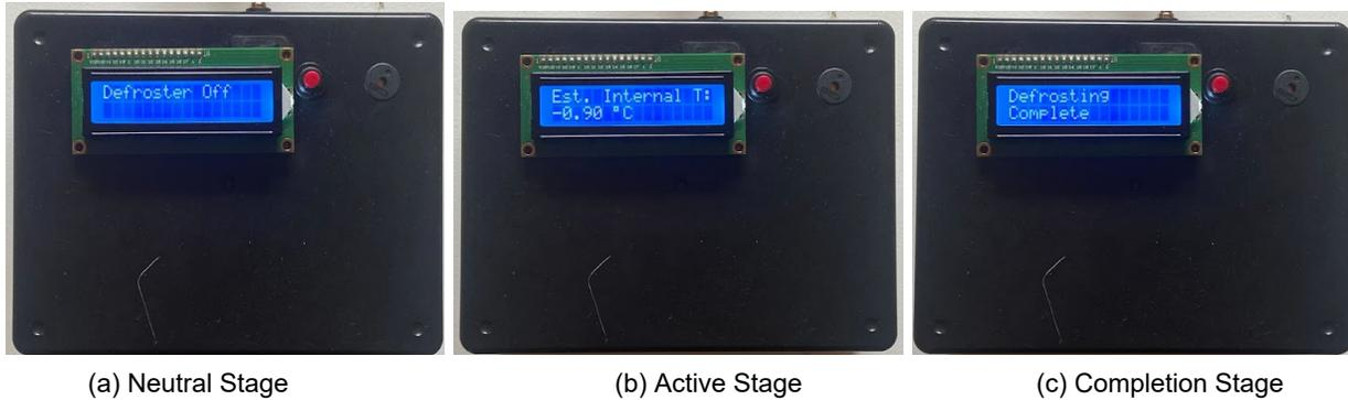
Figure 8: Each Status Stage of the LCD Display.
