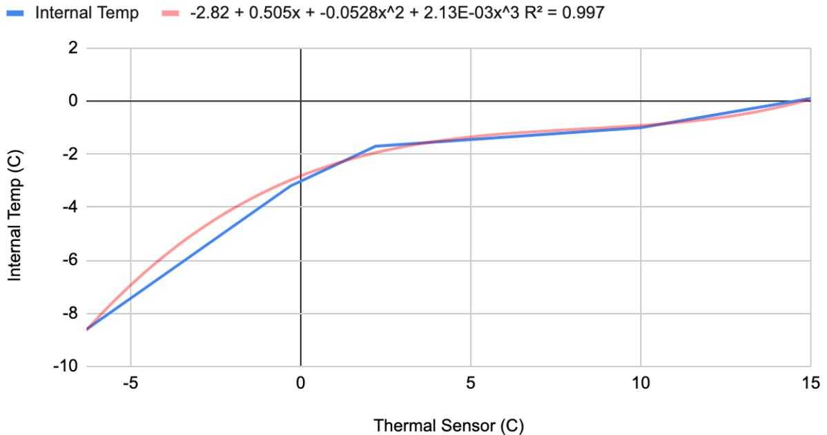
Figure 12: Thermal Sensor to Internal Temperature Poly Regression Line
