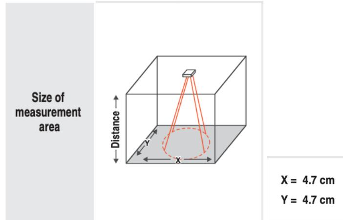
Figure 5: Diagram of the thermal sensor detection radius based on distance
