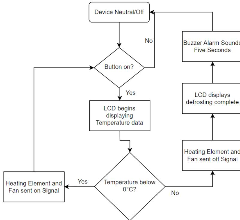
Figure 4: Functional Flow Chart of the Microcontroller Program
