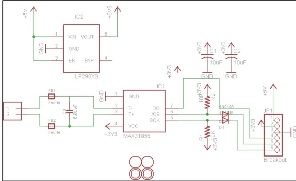
Figure 4: Thermocouple Circuit Design
