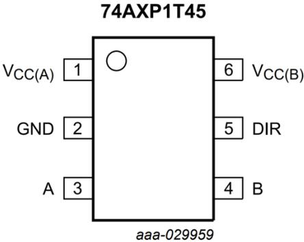
Figure 7: 74AXP1T45 Schematic
