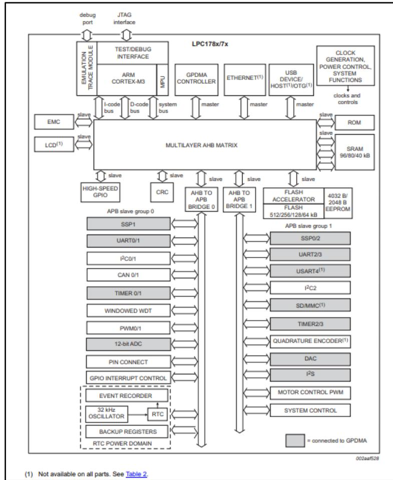
Figure 6: Microcontroller Block Diagram
