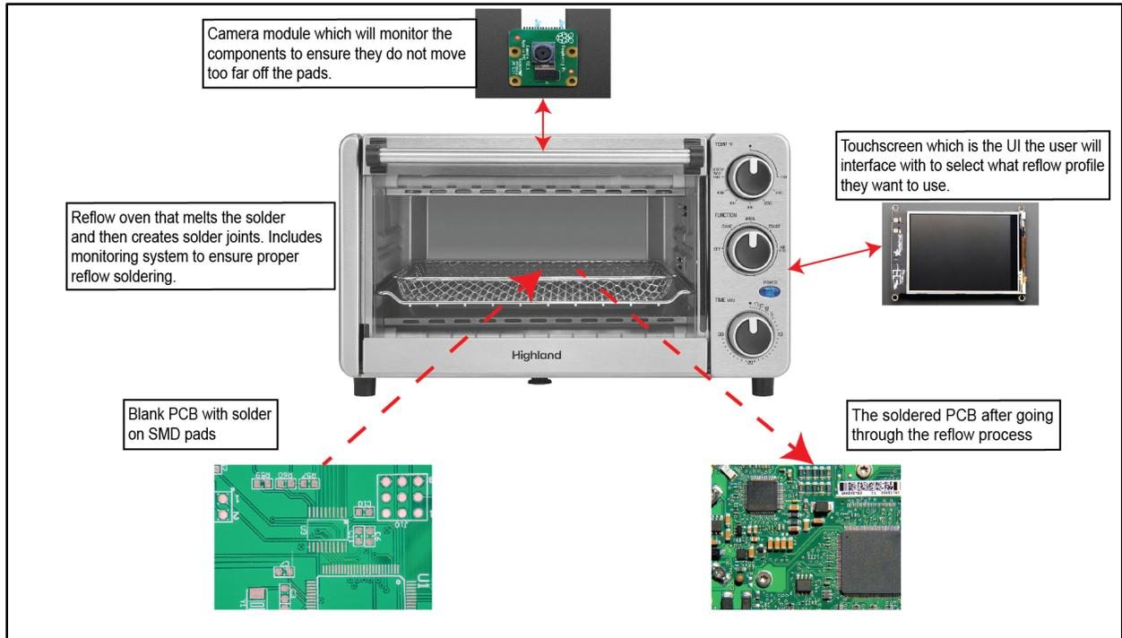
Figure 2: Added features (touchscreen & camera monitoring) our reflow oven will have.
