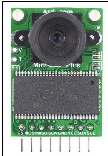
Figure 5: SPI Camera
