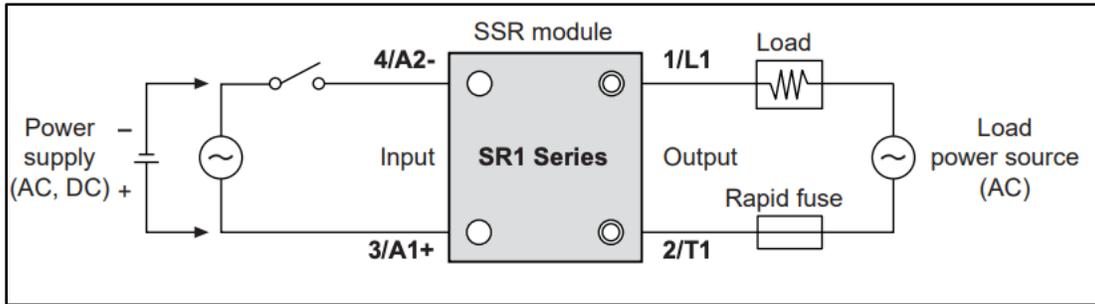
Figure 8: Solid State Relay Circuit
