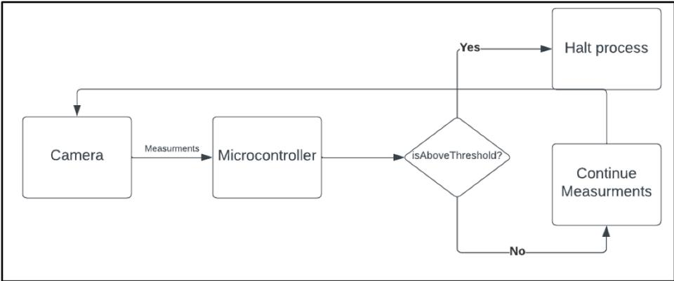
Figure 12: SMD Component Slip Detection
