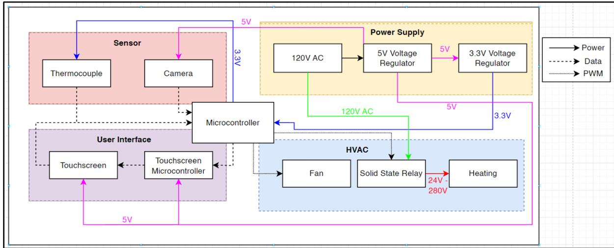
Figure 3: DIY Reflow Oven Block Diagram
