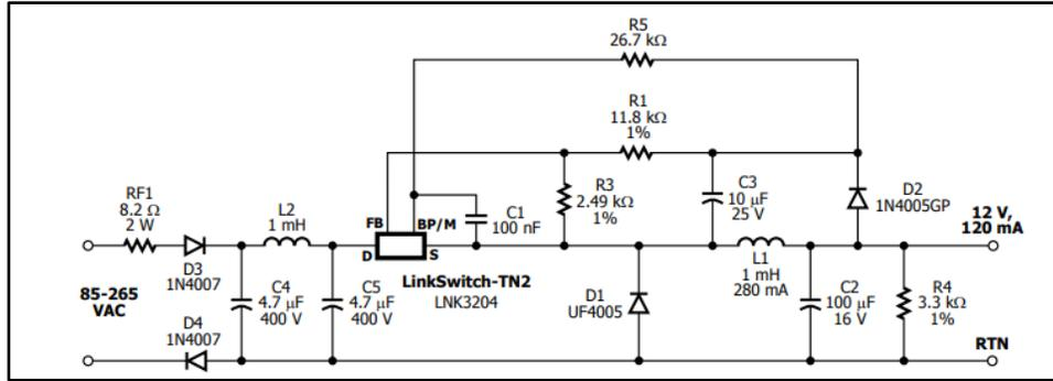
Figure 9: LinkSwitch-TN2 12V Voltage Regulator Circuit
