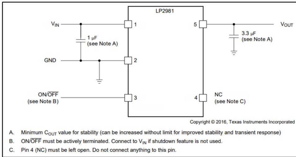
Figure 10: LP2981 Common Application Setup
