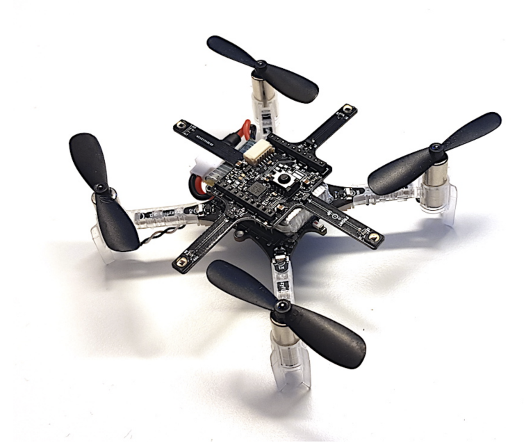
Figure 1. Drone carrying a deck that has an LED-configured PCB [1].
