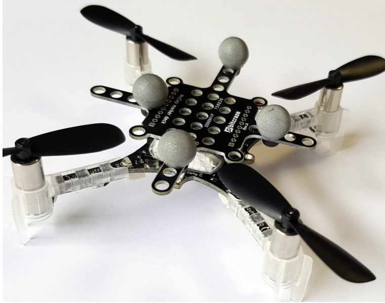
Figure 2. Drone carrying a deck that has holes to attach the reflective balls [1].
