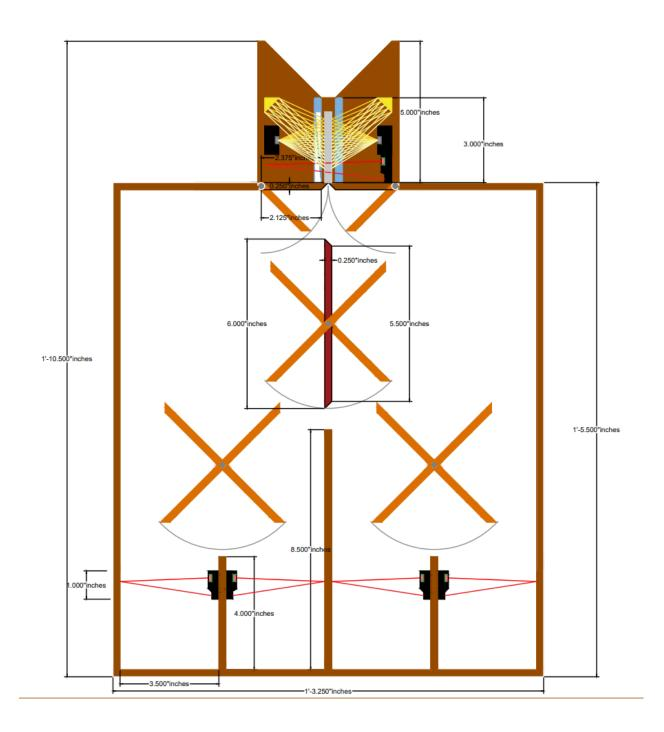
For our physical design, the overall build will be composed of wood with a base dimension of 22.5 inches x 15.25 inches. The front of the apparatus will be covered with a see-through acrylic or plastic to be able to see the workings of the motorized parts and to make debugging much simpler. At the entryway of the mail, there will be a 0.5 inch opening to fit the size of our mail
