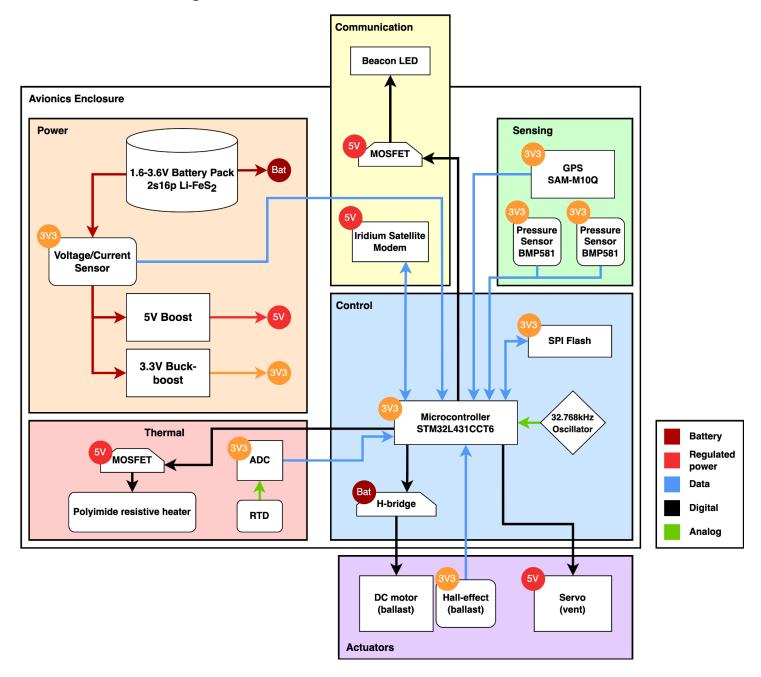
The avionics system is composed of multiple subsystems which perform functions to keep the payload warm, powered, and communicable. The control subsystem is the brains of the avionics, which accepts commands, collects data, and manages the altitude equilibration control loop. The communication subsystem allows for remote data retrieval and commanding via an Iridium
