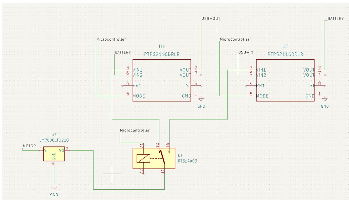
Figure 7. Circuit Schematic for the Hand-Crank Subsystem
