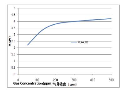
Let **X'** and **Y** be the analog readings from the MQ-3 sensor and a standardized breathalyzer tool, respectively. X will be an analog value 1023. We will map X' to a number between 0V and 5V linearly. Using the data sheet above, we will convert from Volts to ppm, the inverse of which will give us **X** in mg/dL (BAC units). We will then perform the following analysis between **X** and **Y**.
