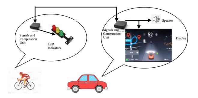
The pictorial representation is depicted above, with arrows indicating data (and computation results) transfer. To summarize, the Signals and Computation Unit of the bike and vehicle work in tandem, to let each other know of their respective positions, finally sending it to the LED indicators, along with the display and speaker respectively. This then informs the user according to specifications mentioned.
