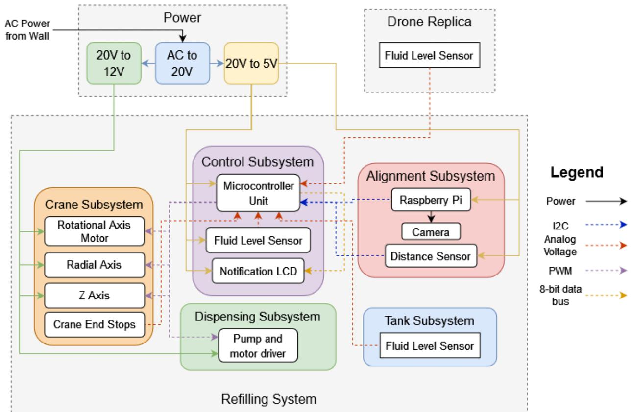
The block diagram shows all of the power connections in addition to the different data connections as shown in various colors in the Legend.
